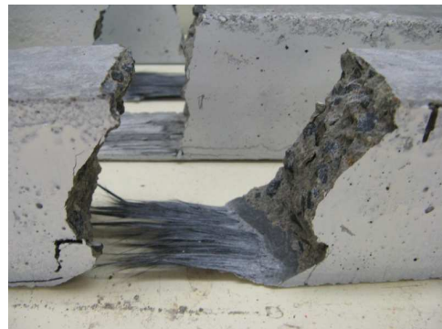
Figure 20 FRP rupture at OSS sample
