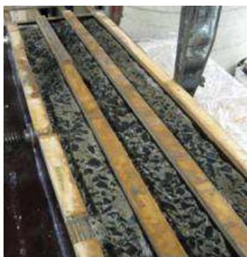
Figure 17 Sandblasted concrete substrate
