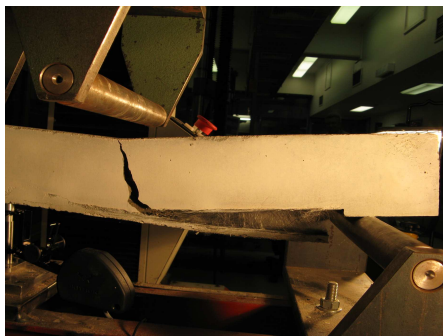
Figure 21 OCS specimen failure
