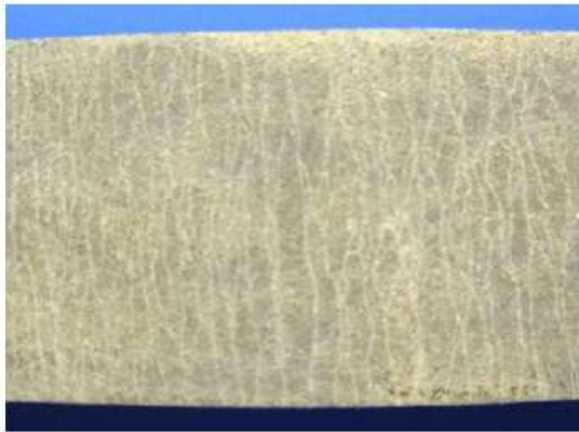
Figure 2. Multiple and micro cracking on the surface of tensile specimen of SDB
