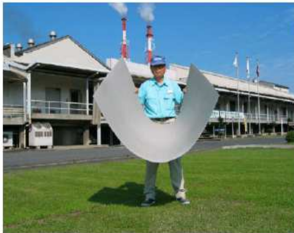
Figure 4 Bendable sheet (2mm thickness)
