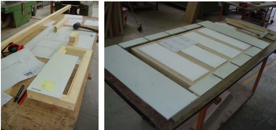
The prototype of the insulated, adjustable shutter finished with fibrecement boards.
