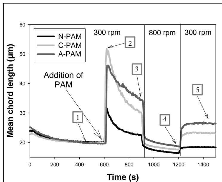
**Figure 2 – Mean chord length evolution with time for 100 ppm dosage of different types of PAM.**
