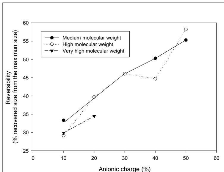
Figure 6 – Effect of molecular weight and charge density on the flock reversibility.
