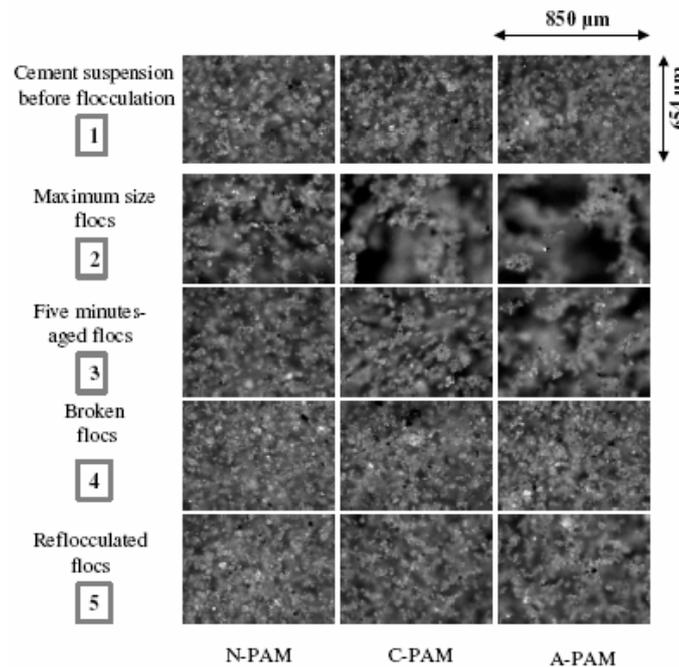
Figure 3 – PVM images evolution with time for 100 ppm dosage of different types of PAM.
