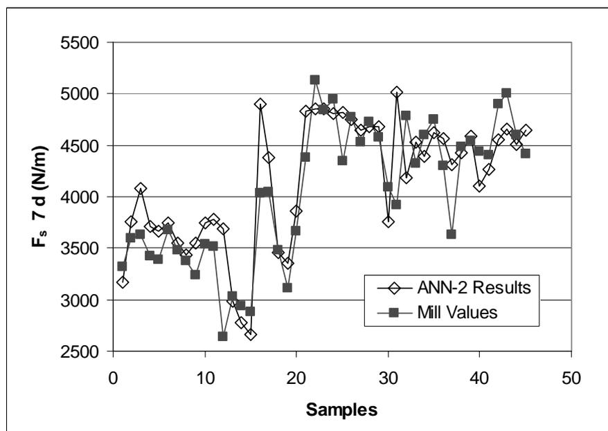
**Figure 9 – Comparison between production data and network results in validation samples for  $F_s$  after 7 days air curing.**
