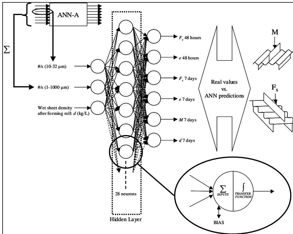
**Figure 10 – Scheme for the carried out work. The main ANN of the scheme could be either ANN-B (one profile) or ANN-C (different profiles).**
