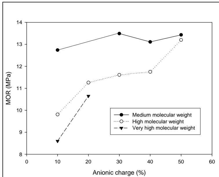
Figure 5 – Effect of molecular weight and charge density of the flocculant on bending strength.
