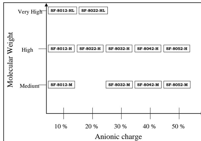
Figure 4 – Anionic charge density and molecular weight of different PAMs.
