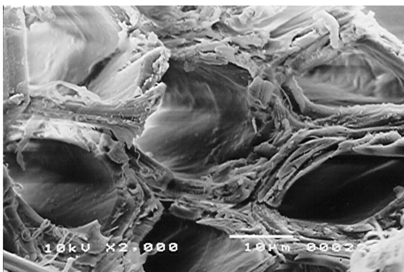
**Figure 1 - Cross section of fique fiber filaments**
