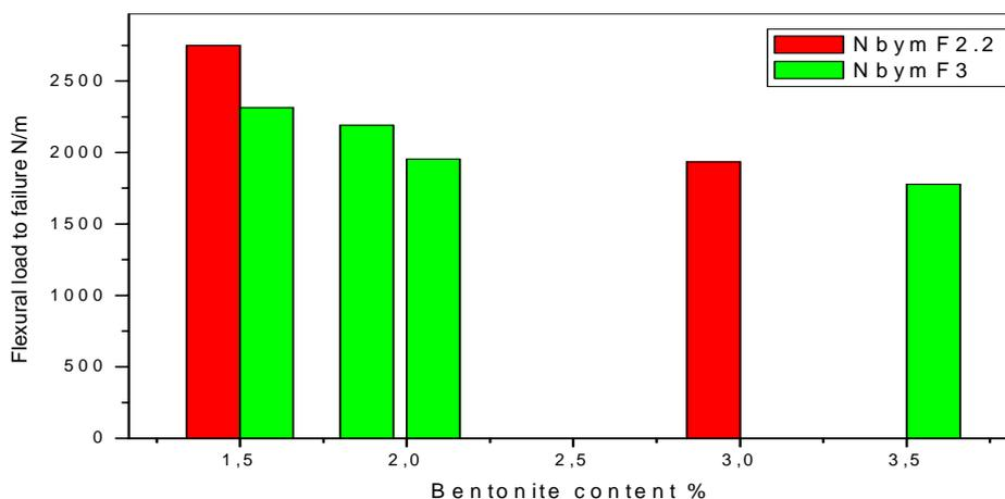
**Figure 6 – Variation of the Flexural load to failure for mixes added with bentonite. Red colored columns represent the mixes reinforced with 2.2% of Figue fibers while the green columns represent the mixes with 3% of fiber.**
