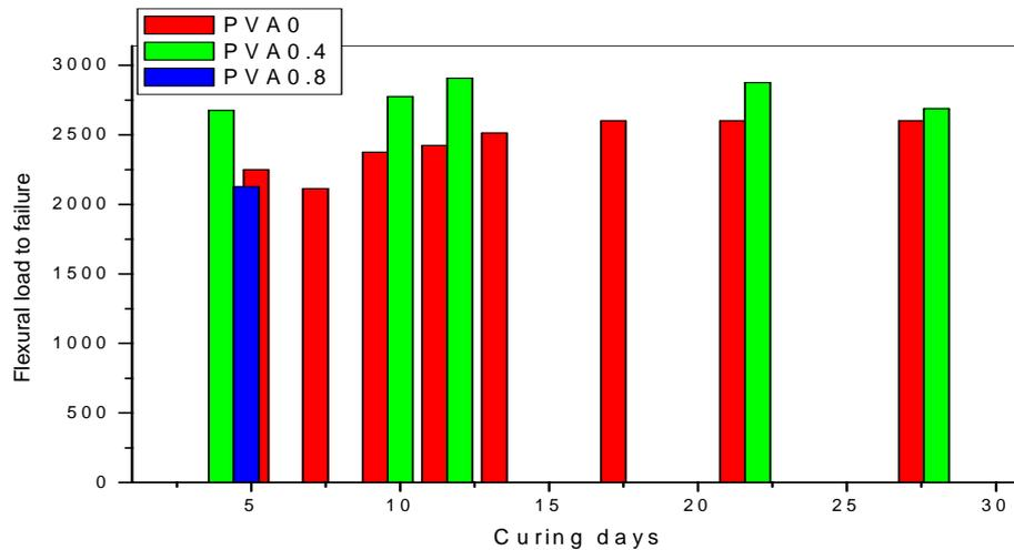
**Figure 7 – Variation of the Flexural load to failure for hybrid mixes reinforced with PVA and fique fibers. Fique fibers amount was fixed at 2.2%.**
