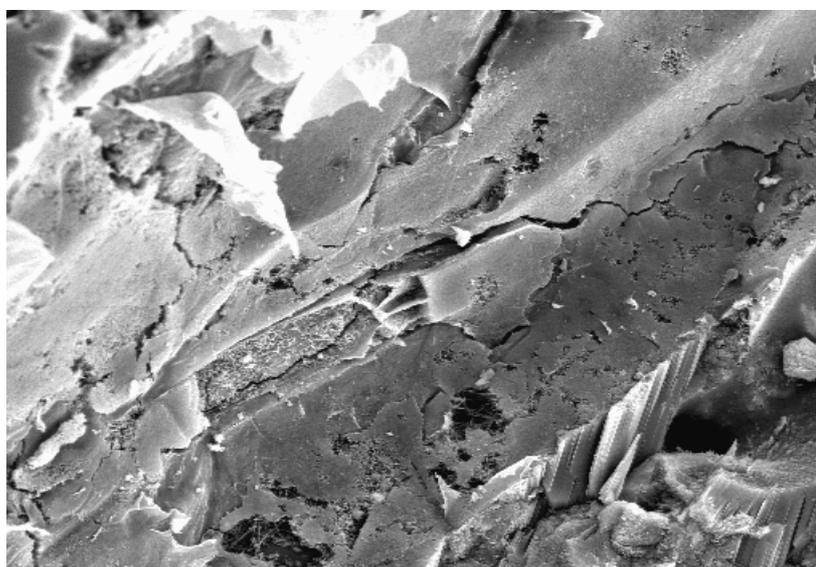
Figure 3 – Face of the cementitious matrix in contact with the Figue fiber (1000 magnifications).
