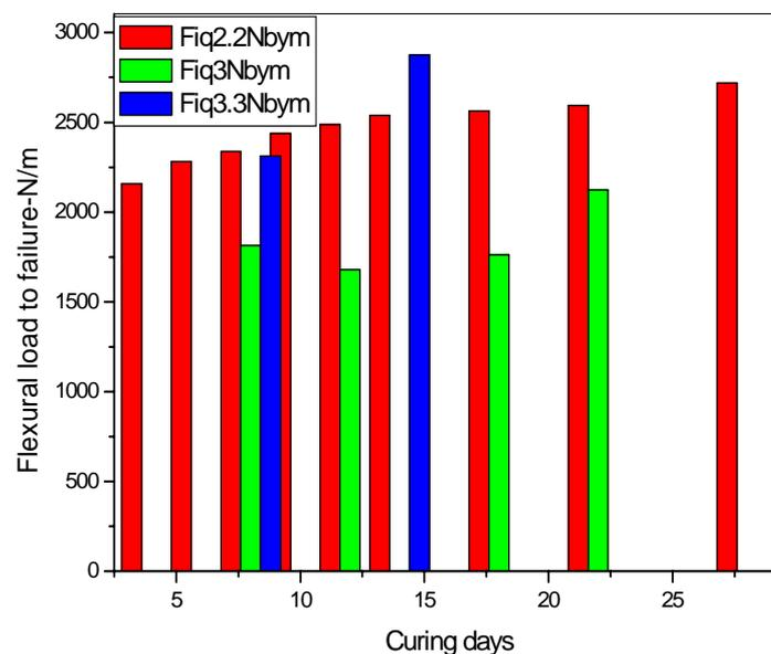
**Figure 4 – Variation of the Flexural load to failure for mixes reinforced with different contents of Fique fiber.**
