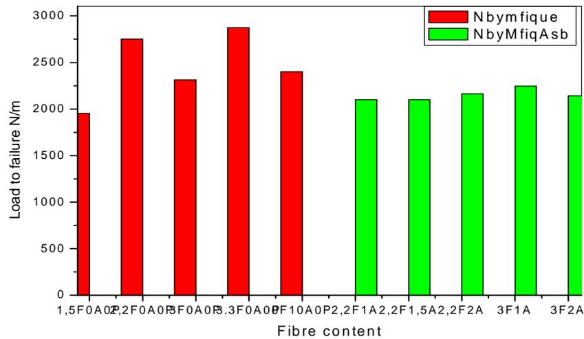
**Figure 5 – Variation of the Flexural load to failure for hybrid mixes reinforced with Figue (red colored) and Asbestos fibers. A letter represents the type of fiber (F for Figue and A for asbestos) and the number after it the % of fiber by weight with respect to the portland cement content.**
