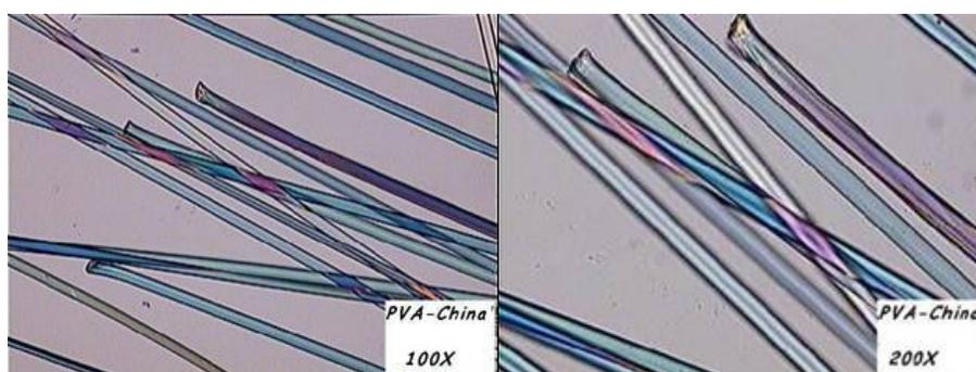
**Figure 10 – Micrographs of commercial PVA (magnification of 100X and 200X)**
