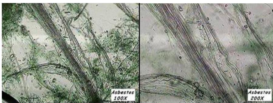
**Figure 9 – Micrographs of asbestos (magnification of 100X and 200X)**
