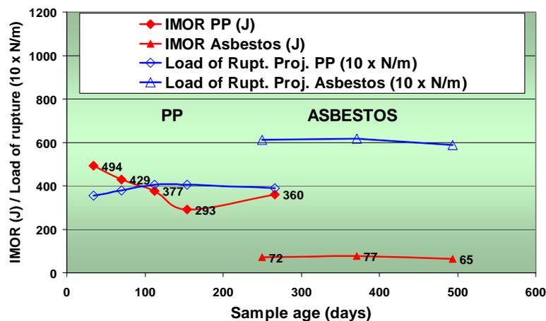
Figure 16 – PP-reinforced and asbestos product comparison of IMOR behavior at early ages
