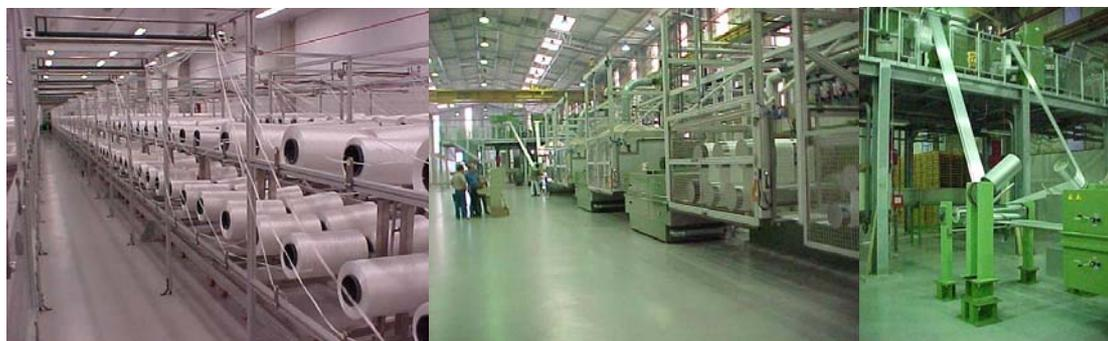
Figure 6 - Drawing/Spin finishing/Cutting stage
