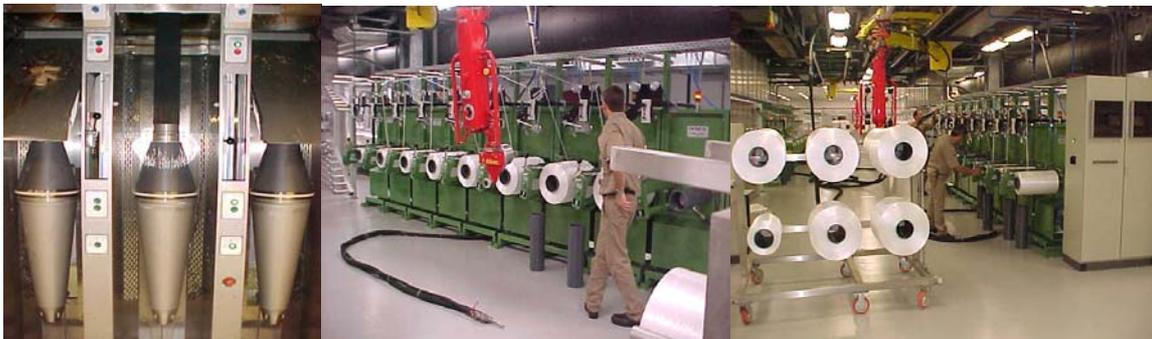
Figure 5 – Spinning and bobbin stage
