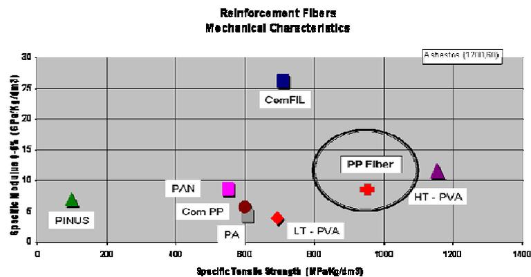
Figure 4 - New Brasifil PP fiber in comparison to commercial alternative fibers. (From Houang, 2001)
