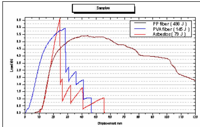
Figure 12 – Comparison curves of breaking load of corrugated sheets with PP Brasifil, PVA and asbestos after conditioning at room temperature (according to EN 494:1994). In parentheses, the calculated total energy to break (in Joules).
