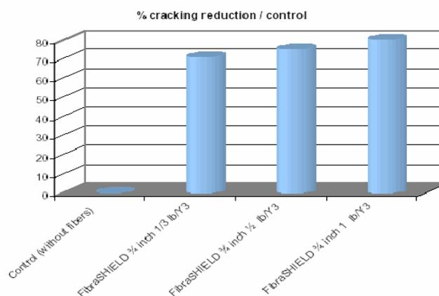
**Figure 18 – Percentage of cracking reduction using FibrashIELD®Mono anticrack High tenacity PP fiber.**
