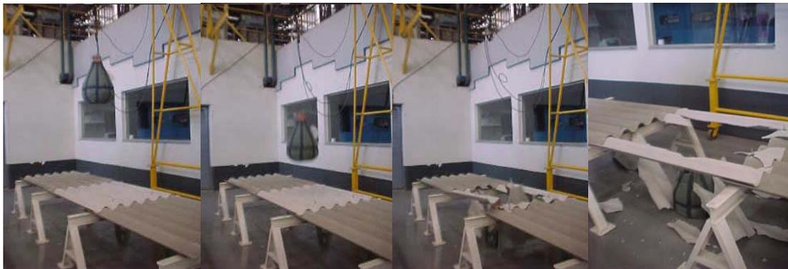
**Figure 15 – Impact resistance test (600 J) of asbestos corrugated sheet P7 – 6mm.**
