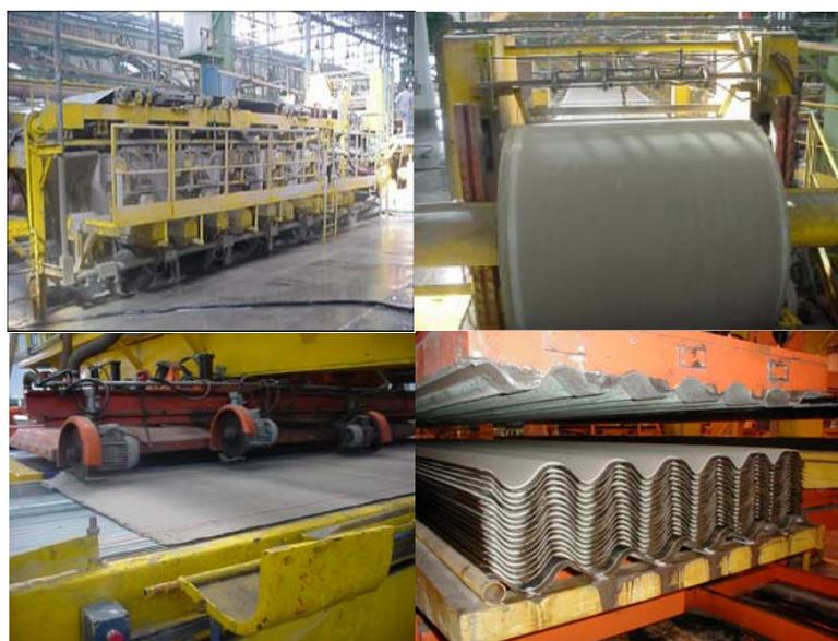
**Figure 1 – General view of Hatschek machine, pressing roll, cutting system and corrugating process.**
