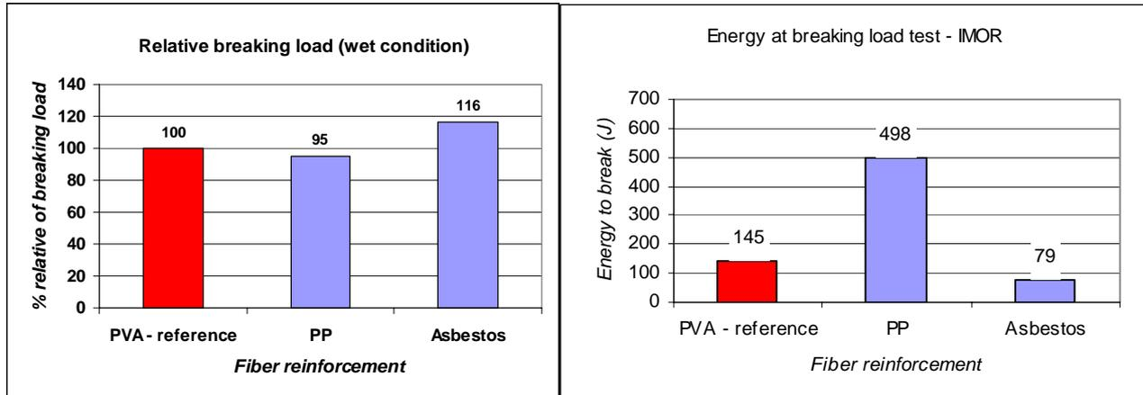
**Figure 13 – Example representative of relative breaking load under wet condition and the IMOR-energy to break of PP and asbestos corrugated sheets in reference to PVA.**
