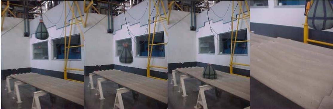
**Figure 14 – Impact resistance test (600 J) of corrugated sheet P7 – 6 mm using Brasifil.**
