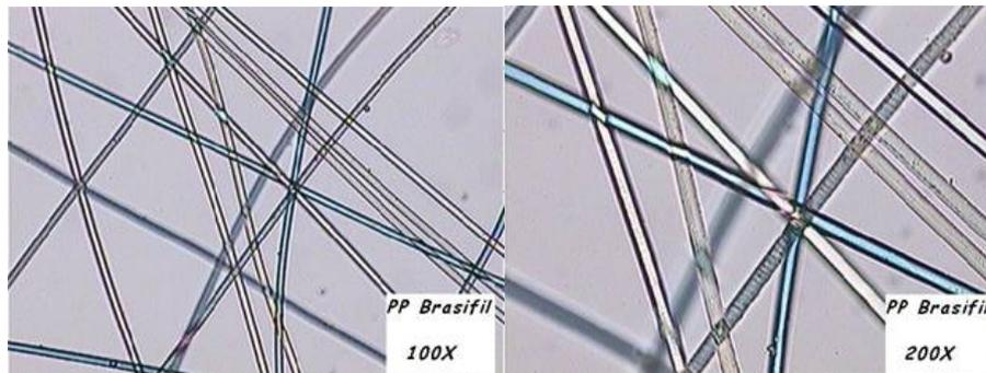
Figure 11 – Micrographs of PP Brasifil (magnification of 100X and 200X)
