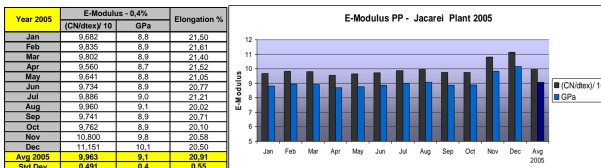
**Figure 8 – Quality data for mechanical properties.**
