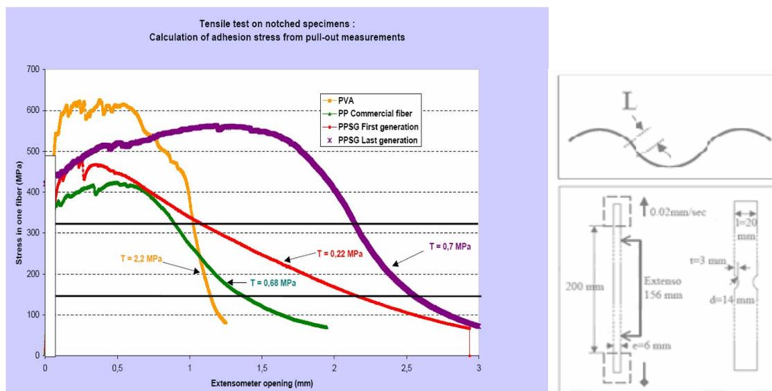
**Figure 4 – Testing procedure diagram and comparison between commercial PP and PVA to surface treated PP’s fiber developed by Saint-Gobain—CRM / Brasilit. (From Morlat, 2001)**
