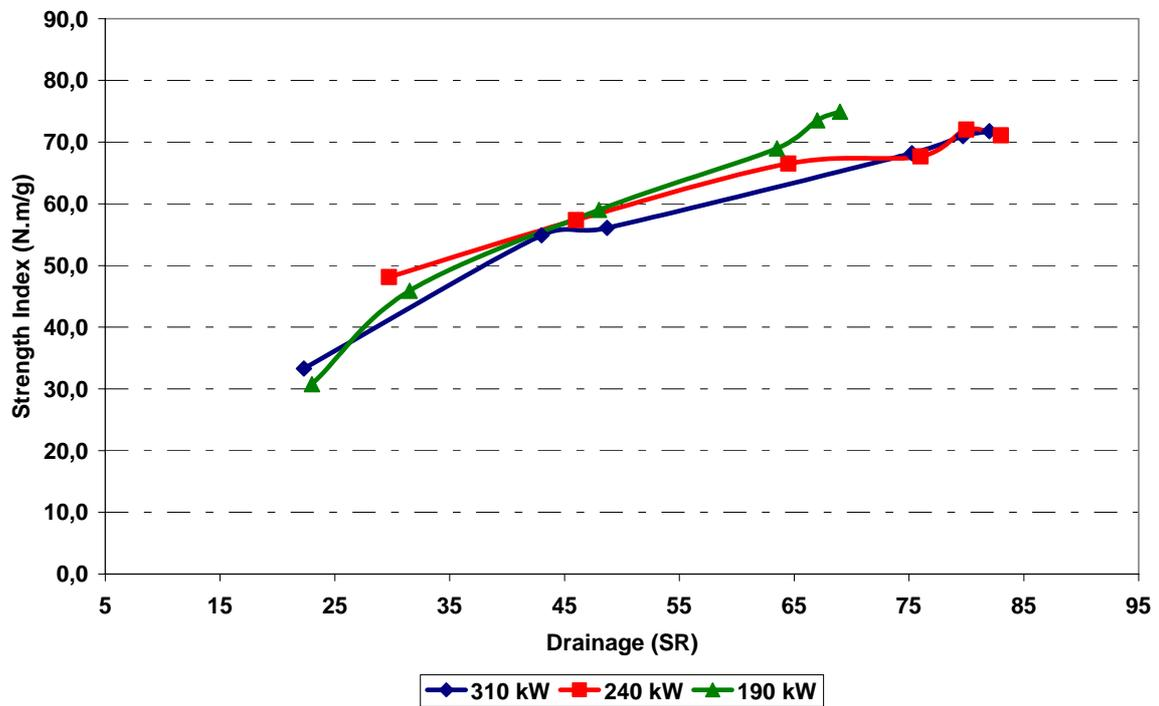
**Figure 2 – Drainability versus Strength Index at different power levels for Eucalyptus Fibre.**
