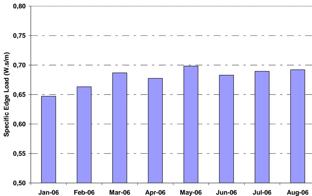
Figure 5 – Specific Edge Load during 2006 Industrial Production.
