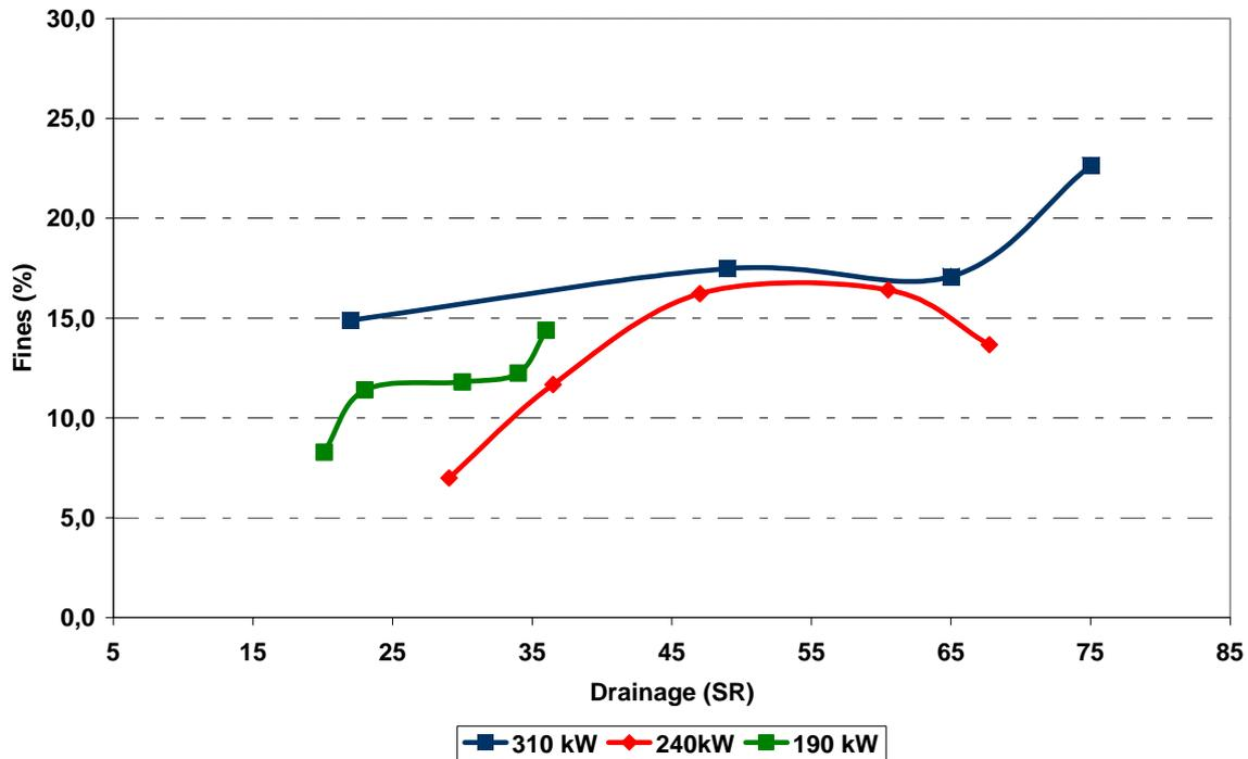
Figure 3 – Drainability versus Fines Content at different power levels for Long Fibre.
