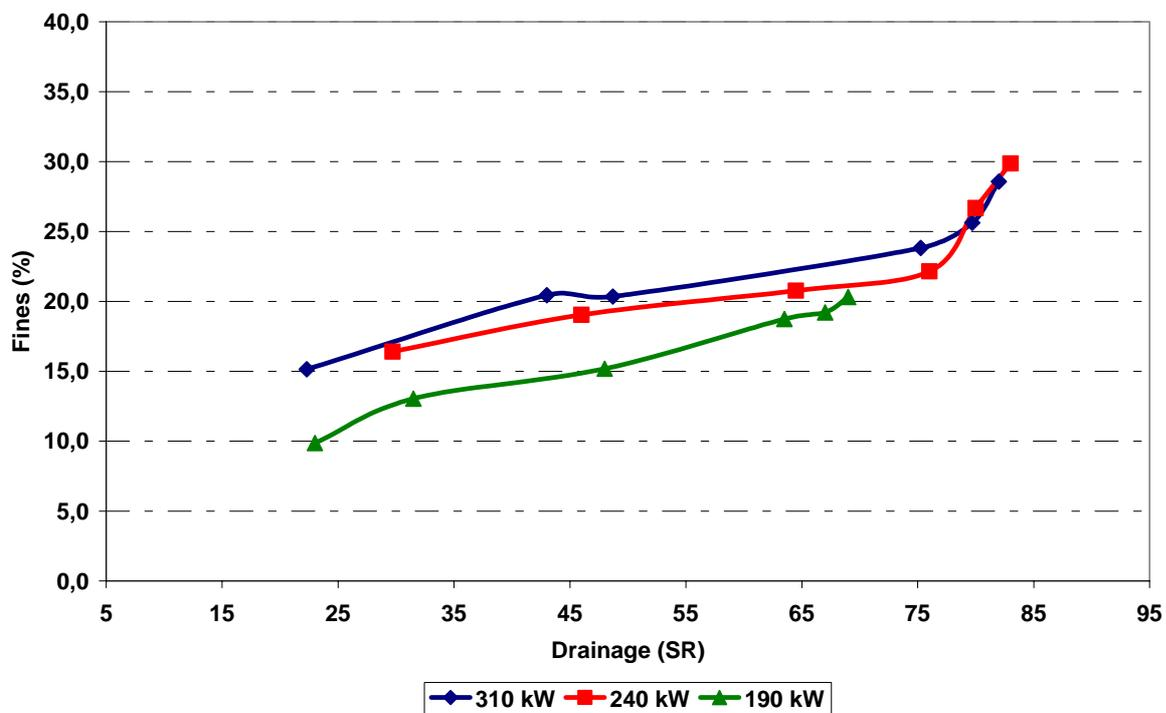
Figure 4 – Drainability versus Fines Content at different power levels for Eucalyptus Fibre.
