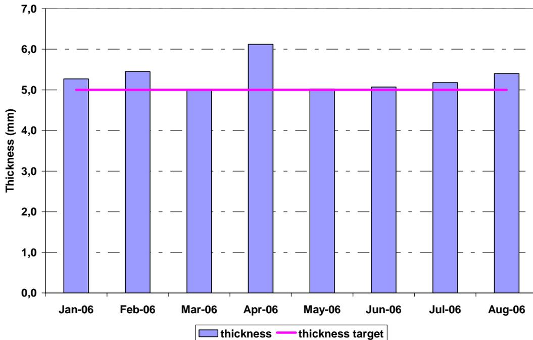
**Figure 8 – Corrugated fibreceement roofing thickness.**
