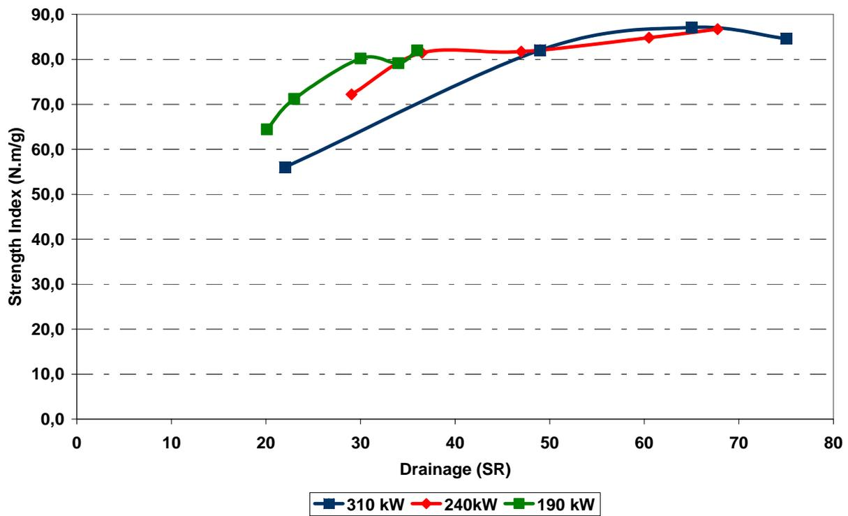
Figure 1 – Drainability versus Strength Index at different power levels for Long Fibre.
