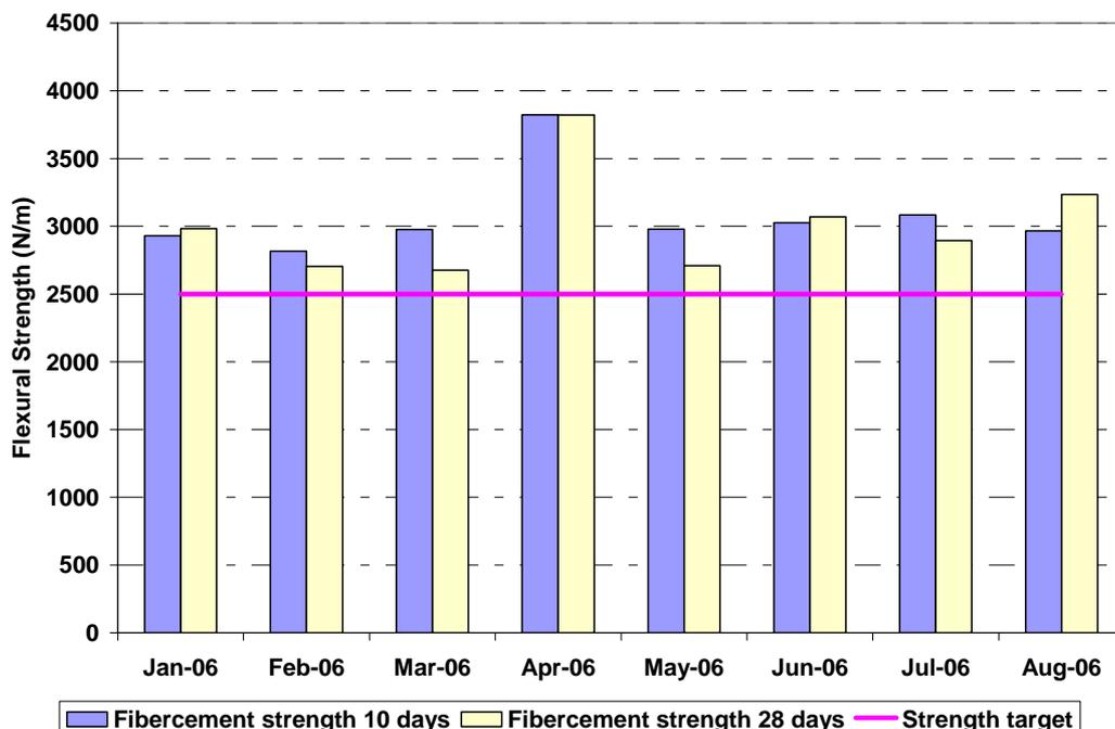
**Figure 9 – Corrugated fibreceement roofing Flexural Strength.**
