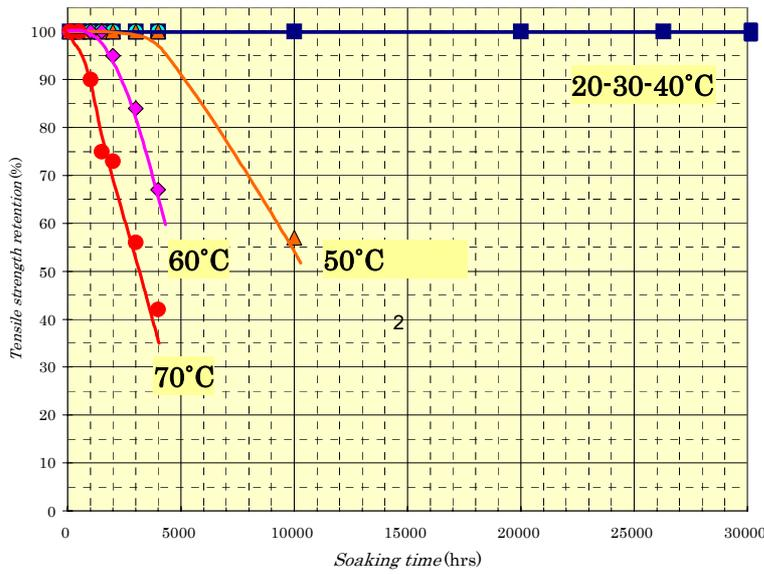
Figure 1. Effect of the soaking time on the tensile strength retention
