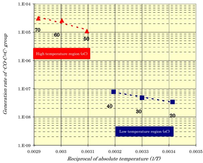
Figure 7. Dependence of the generation rate of ·CO·C=C· group on temperature (Arrhenius plot)
