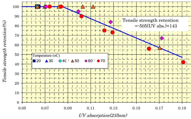
Figure 4. Relation between the tensile strength retention and UV absorption
