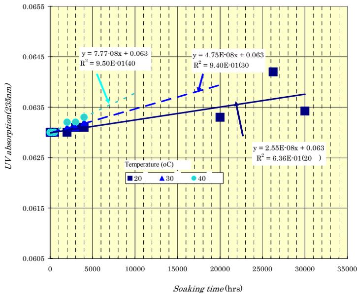
Figure 6. Relation between UV absorption and soaking time mesurded below 40
