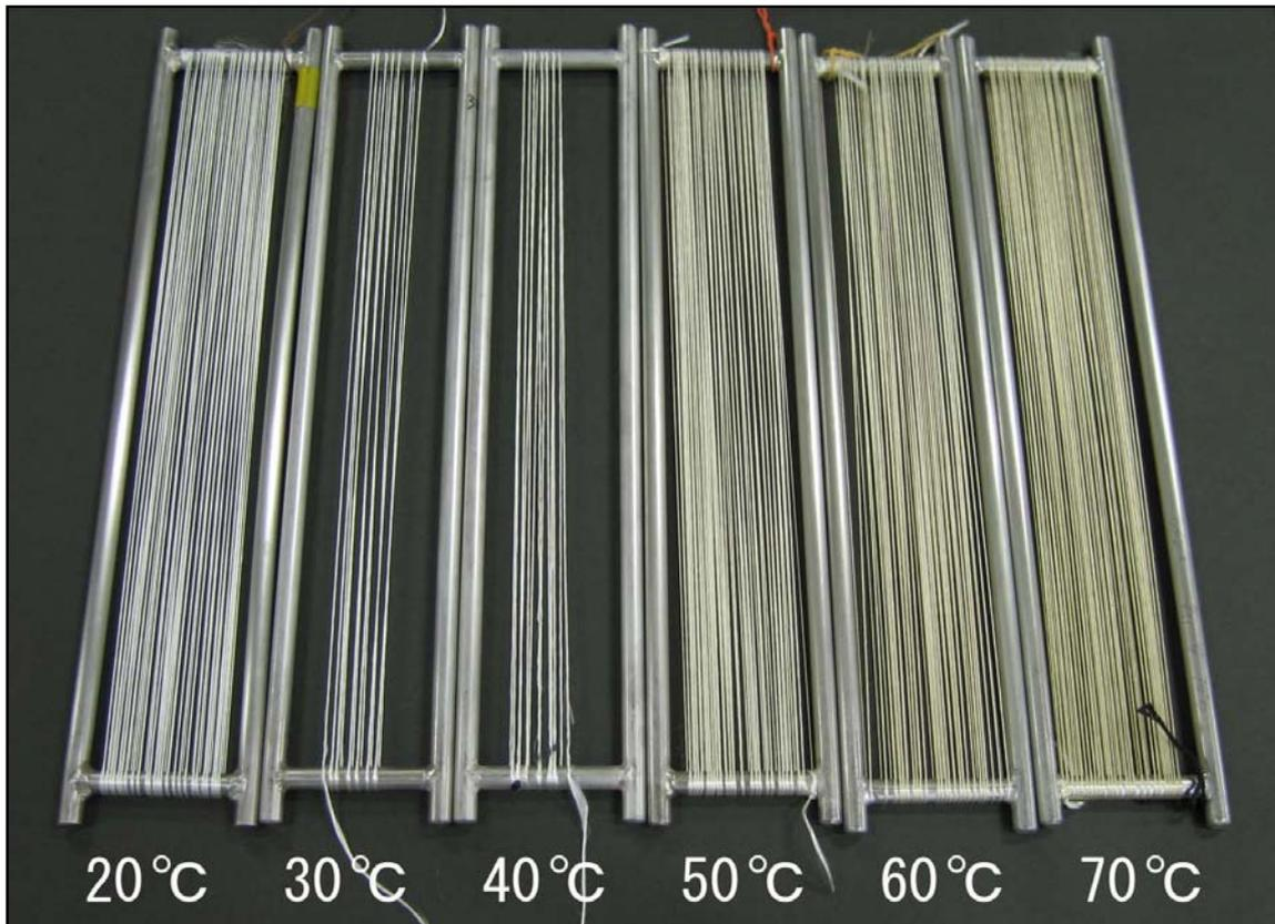
Frames used for soaking yarn into alkaline solution
