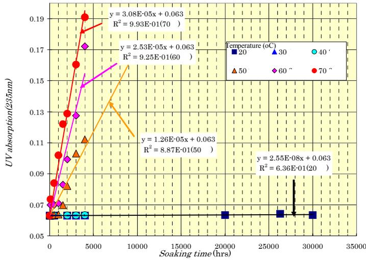
Figure 5 Relation between UV absorption and soaking time
