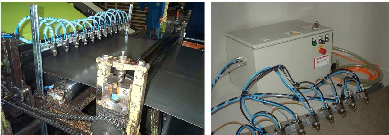
Figure 3 – SYRO Oiling System HB2000 in use with a coil system
