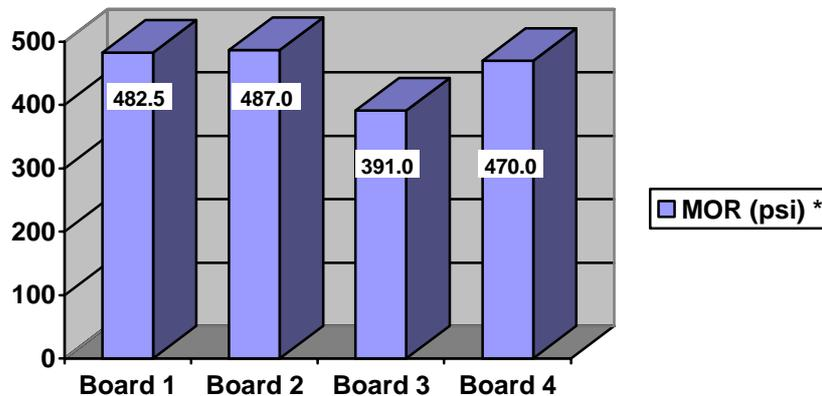
Figure 4: Modulus of rupture (\*properties were obtained from specimens with short spans, so some small reduction due to shear effects may be presumed)
