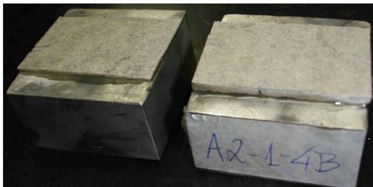
**Figure 6: Delamination after pull off.**
