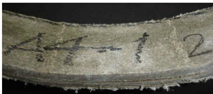
**Figure 4: Delamination after bending.**
