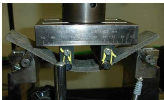
**Figure 3: 4-point bending.**
