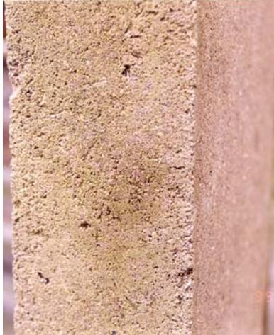
Surface straw particles fall out of the StrawCrete material after prolonged exposure to British weather.
