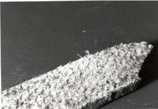
Asbestos cement corrugated sheeting demonstrating fall out of asbestos fiber.
