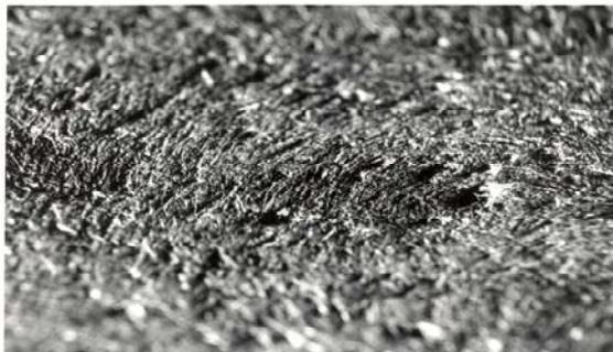
Asbestos cement cladding demonstrating asbestos fibre fallout in old materials
