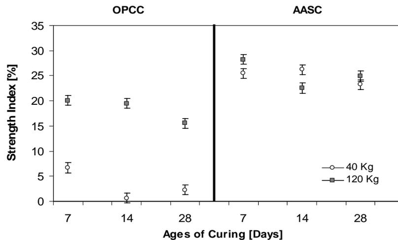
**Figure 1 - Compressive Strength Index of Concrete**
