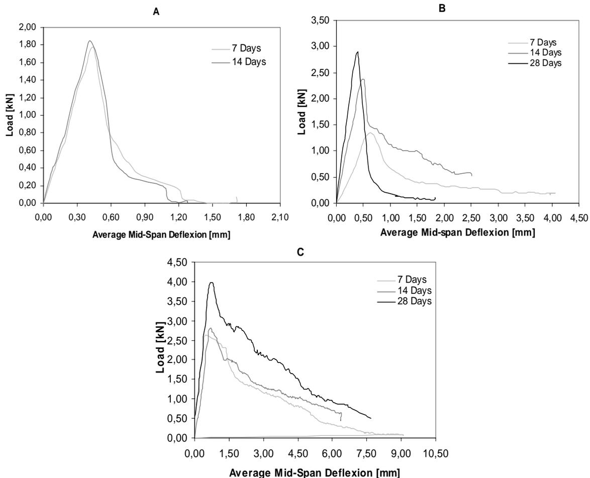
Figure 5- Flexion Strength of Geopolymeric Concretes in Notched Specimens with (A) –  $0 \text{ Kg/m}^3$ ; (B) –  $40 \text{ Kg/m}^3$  and (C) –  $120 \text{ Kg/m}^3$  of fiber incorporated, respectively.
