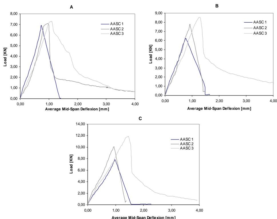
**Figure 2- Flexural Behavior of Gepolymeric Concretes at (A) – 7 Days; (B) – 14 Days and (C) – 28 Days of curing, respectively.**
