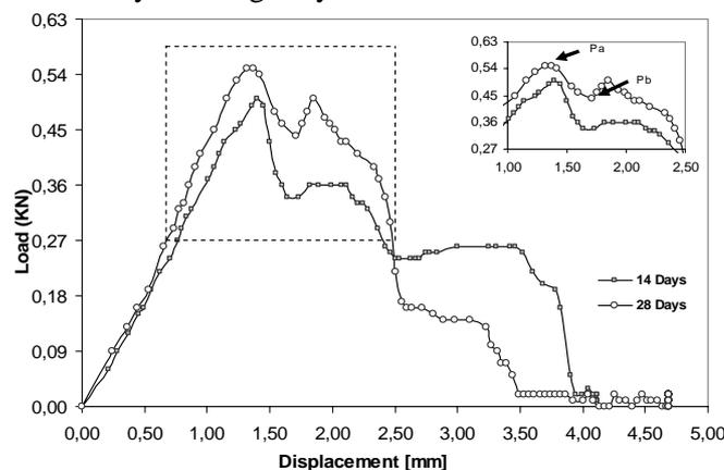
**Figure 4 – Pullout Curves of Geopolymeric Matrix of Concrete**
