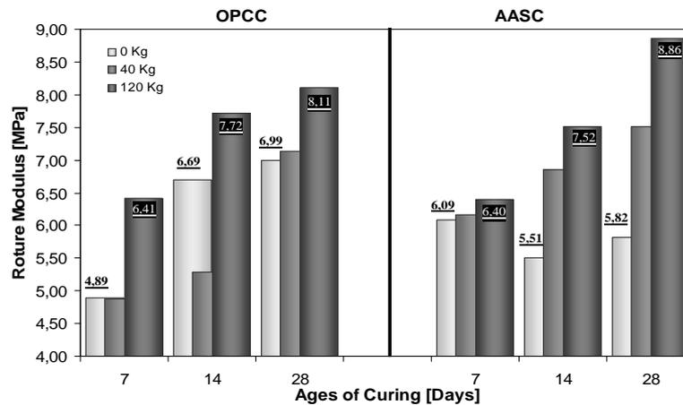
**Figure 3- Modulus of Rupture (MOR) of the OPCC and the AASC**
