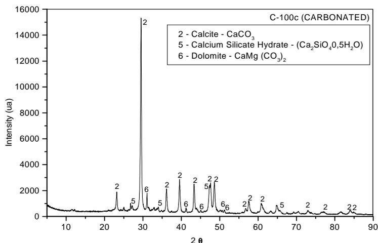
**Figure 5 – X-ray diffraction pattern of the carbonated tiles after 100 ageing cycles.**
