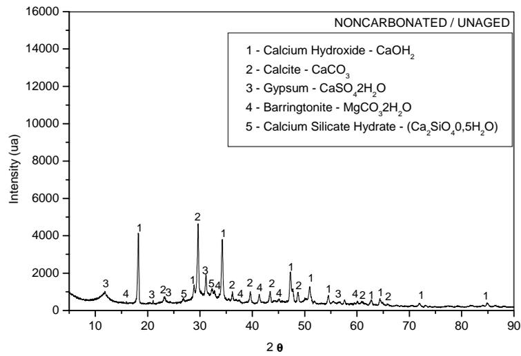
Figure 3 – X-ray diffraction pattern of the unaged and noncarbonated tiles.
