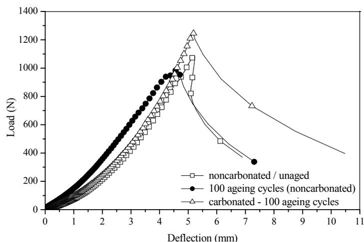
**Figure 2 – Load-deflection curves for the tiles of the different treatments.**
