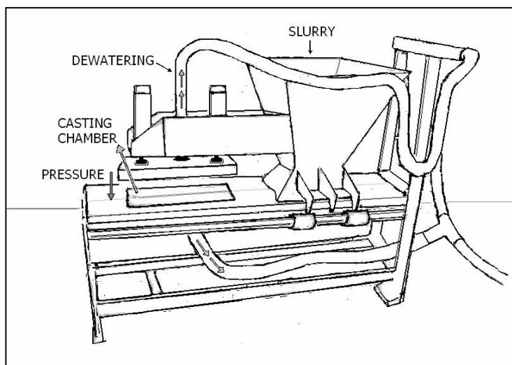
**Figure 1 – Schematic view of the semi-automated device used for roofing tiles molding.**
