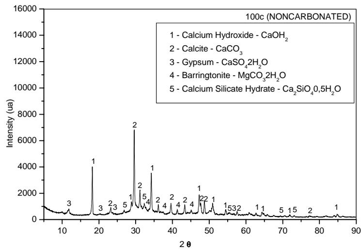
Figure 4 – X-ray diffraction pattern of the tiles after 100 ageing cycles (noncarbonated).
