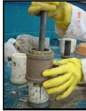
Figure 2 - Compaction in the cylindrical
