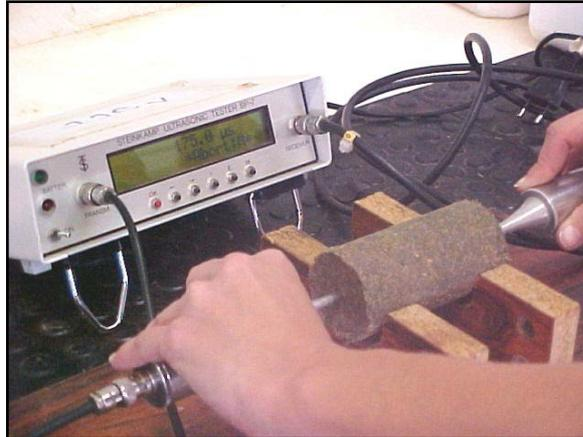
Figure 5 – Ultrasonic tester Steinkamp model BP7
