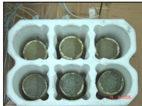
Figure 4 - cylindrical moulds with PT 100
