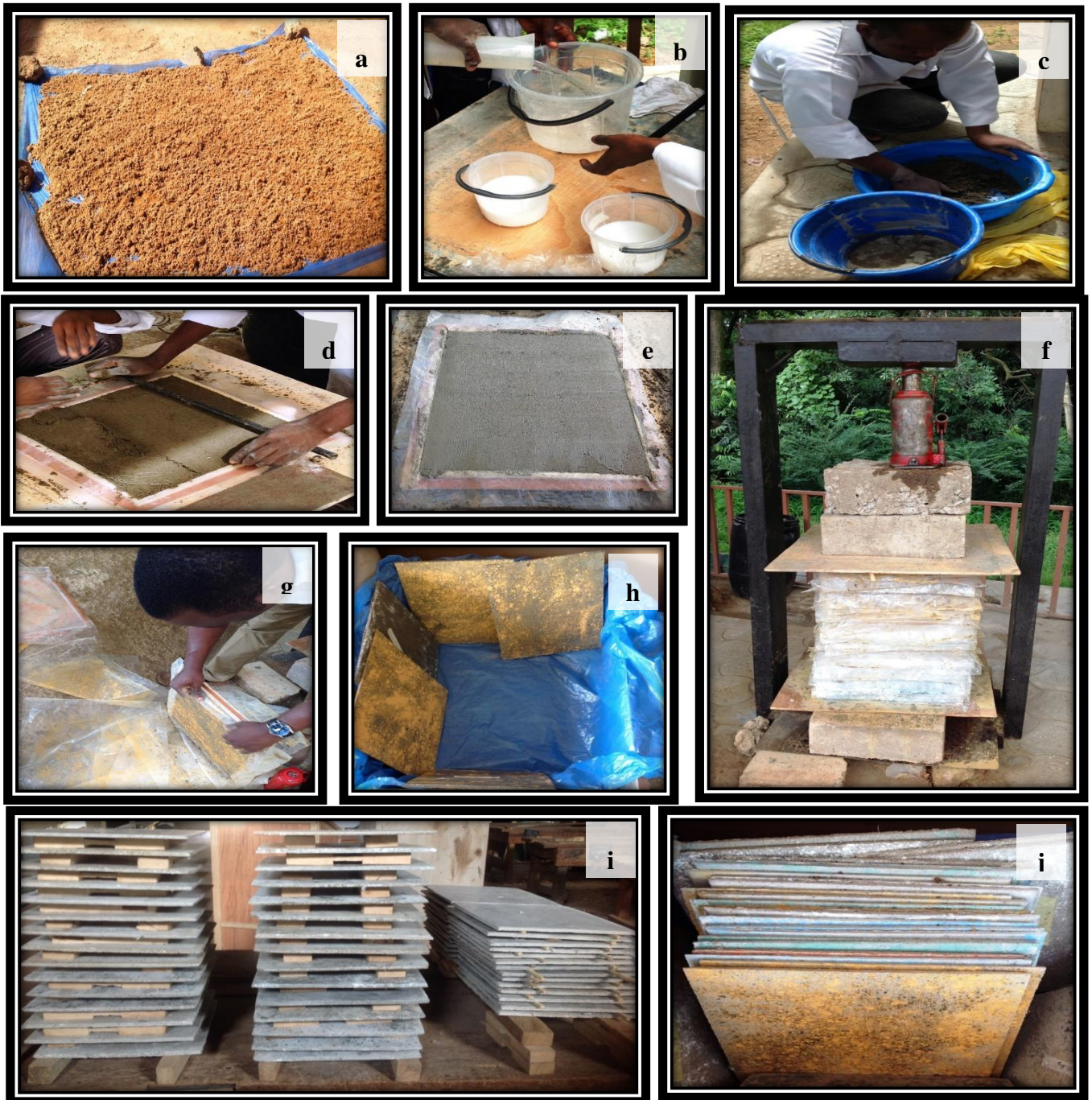
Plates 1 (a) Drying of the bamboo dust; (b) Dissolving of additive (Calcium chloride) for mixture with particle mix; (c) Homogenous mixing of the particle/cement binder/CaCl 2 mix; (d) Flattening of the composite board; (e) Semi-finished cold pressed bamboo cement composite; (f) Cold pressing of the moulded bamboo cement composite at 1.23N/mm 2 pressure; (g) Demoulding of the bamboo cement composite; (h) Conditioning of the bamboo cement composite after demoulding for post curing; (i) Air drying of the bamboo cement composite; and (j) Cement Bonded Particle Boards Produced
