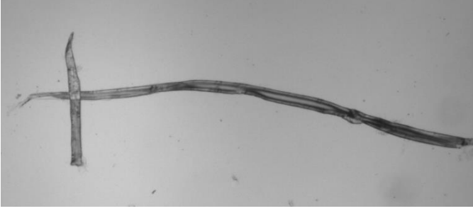
Figure 4 – Contrast of typical short cutting fiber (vertical) and normal fiber (horizontal) observed by microscope.
