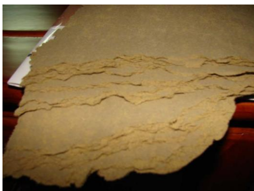
Figure 7 – Typical boards with separated fiber layers and cement layers.
