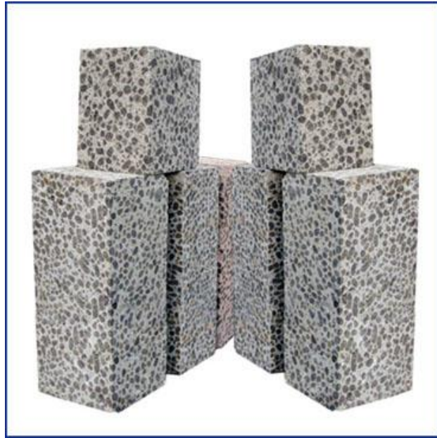
Figure 5: Light weight concrete for using Keramzit [3]
