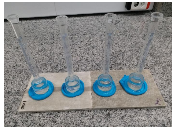
Figure 3 – Illustration of Rilem test (Karsten tube affixed on boards and filled with water)
