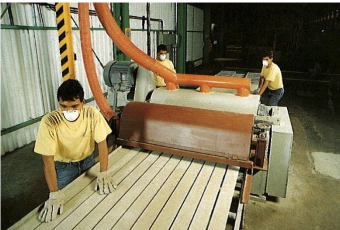
The fibre cement boards are cut into strips. These serve to connect the individual house elements.
