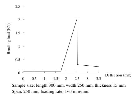
Figure 4— Relationship between bending load and deflection of the extruded CCA sample
