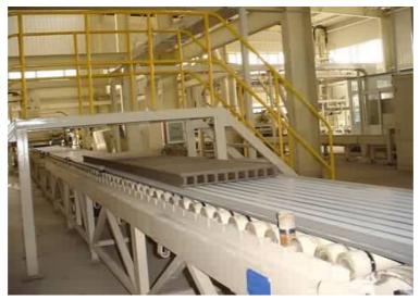
Figure 6—A hollow panel on the conveyor after extruding and cutting
