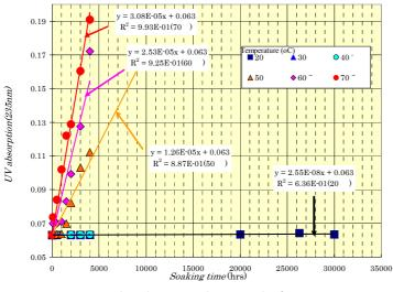
Figure 5 Relation between UV absorption and soaking time
