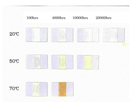
Figure 2. Fiber discoloration due to soaking in alkaline water
