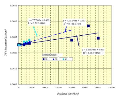
Figure 6. Relation between UV absorption and soaking time mesurured below  $40\,$
