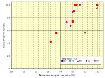
Figure 3. Relation between the tensile strength retention and the molecular weight retention
