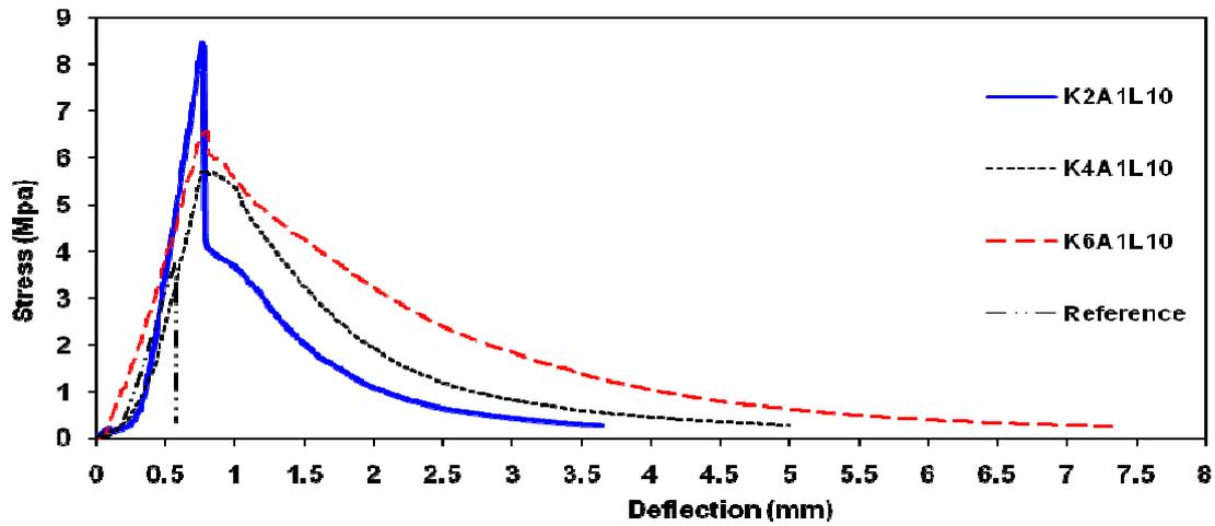
Figure 5 - Stress vs. deflection for specimens with 1% Acrylic fibres.
