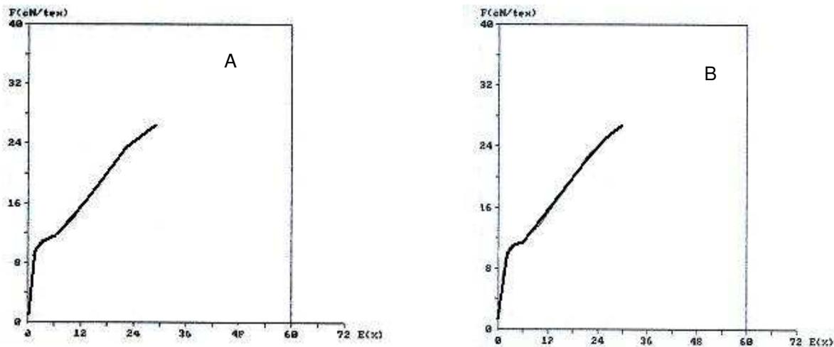
Figure 3 – Tensile test results for Acrylic fibre before (A) and after (B) submerging in alkaline solution.
