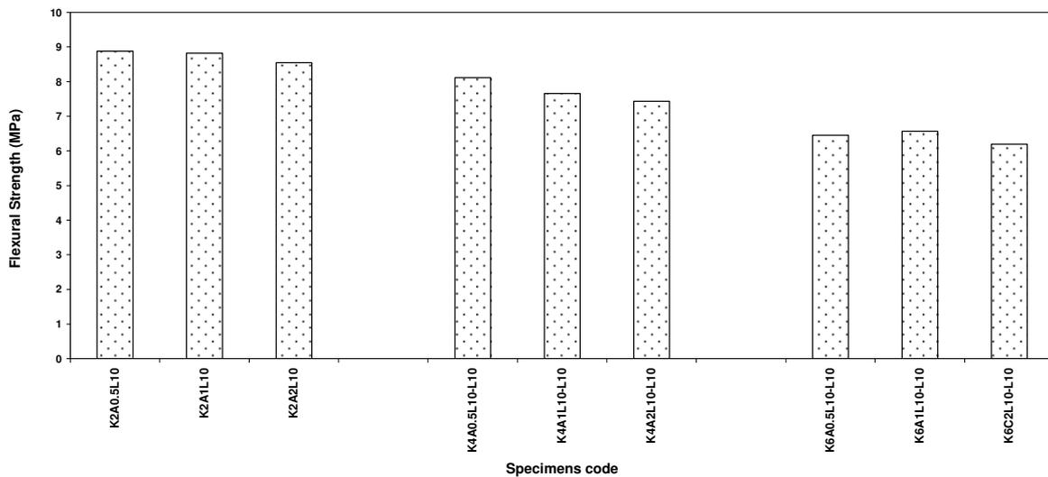
Figure 11 – Maximum flexural strength of the blended fibres cement composite sheets.
