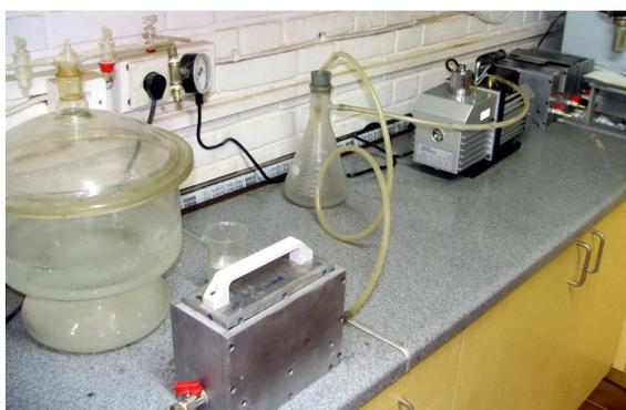
**Figure 1 – The mould and the vacuum set up used to cast the cement boards.**
