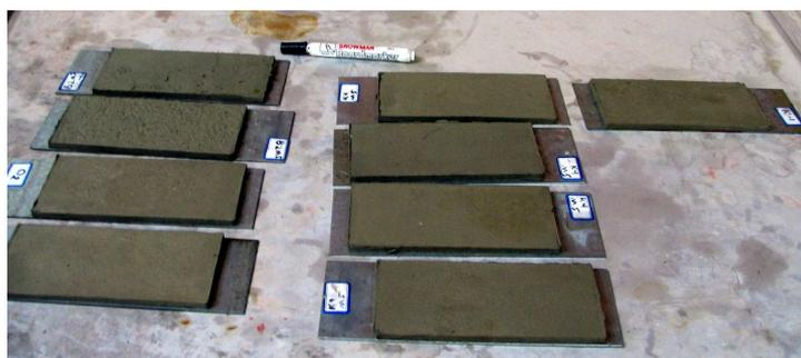
**Figure 2 - The fresh composite cement board specimens after casting.**
