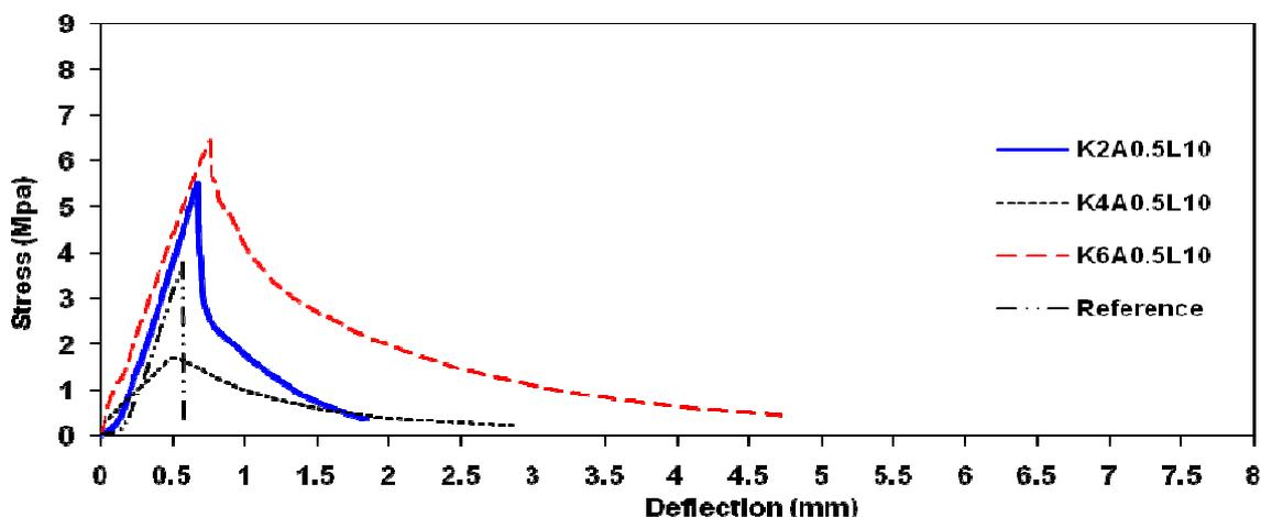
Figure 4 - Stress vs. deflection for specimens with 0.5% Acrylic fibres.
