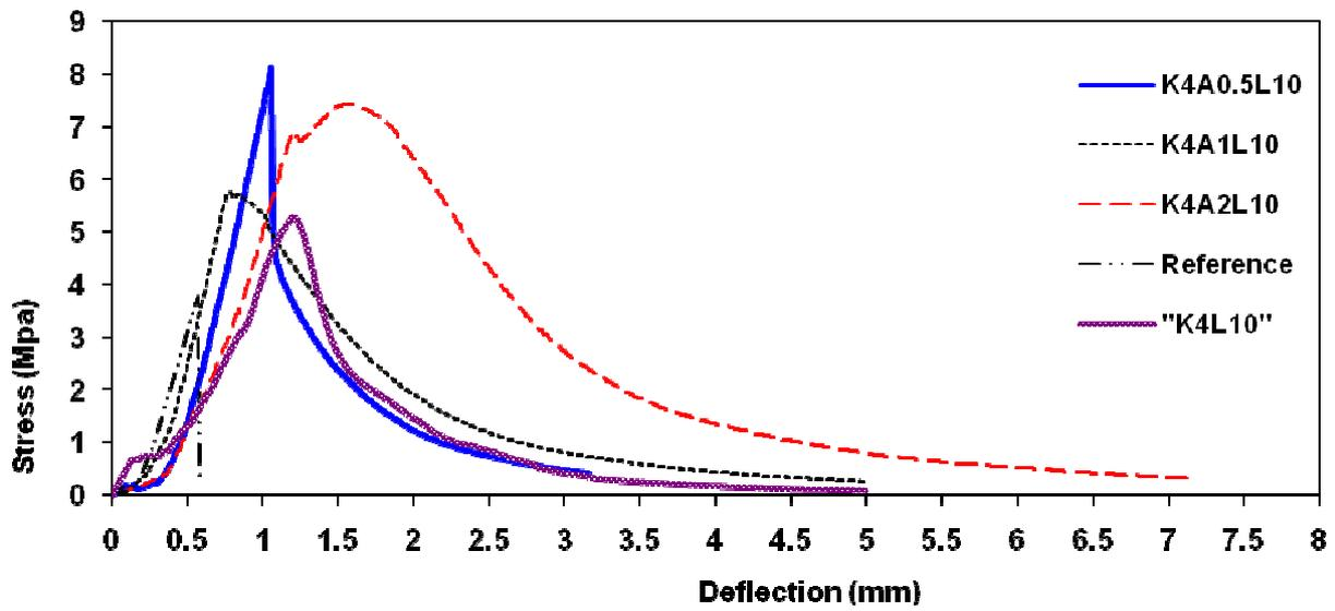
Figure 8 - Stress vs. deflection for specimens with 4% Kraft fibres.
