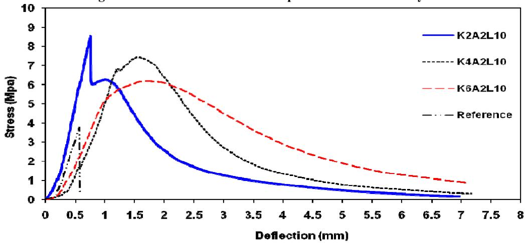
Figure 6 - Stress vs. deflection for specimens with 2% Acrylic fibres.
