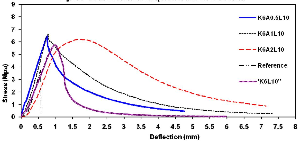
Figure 9 - Stress vs. deflection for specimens with 6% Kraft fibres.
