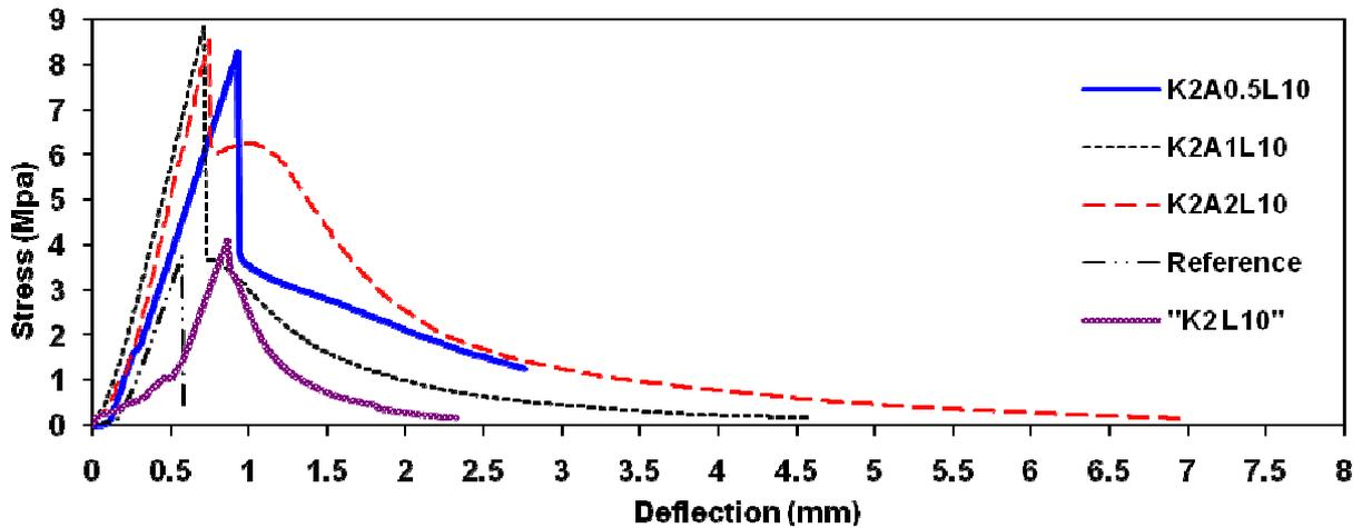
Figure 7 - Stress vs. deflection for specimens with 2% Kraft fibres.
