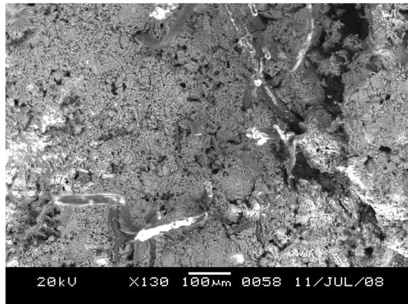
Figure 12 – Smooth surface and uniformly distributed fibres in the fractured surface of the K2A1L10.
