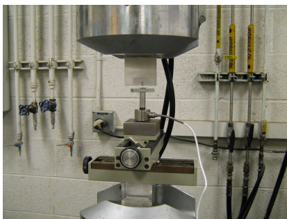
Fig. 12 – Pullout single fibre test setup
