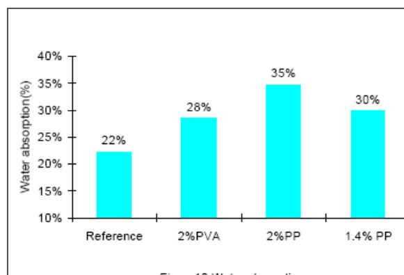
Figure10 Water absorption
