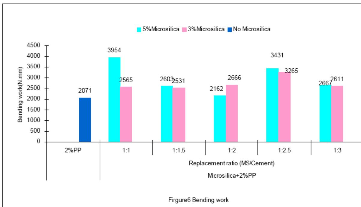
Figure 6 Bending work
