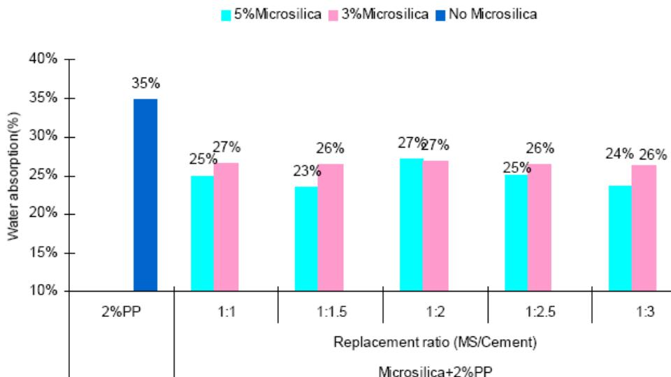
Figure4 Water absorption
