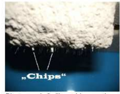
Photograph 3, fibre chips partly dispersed
