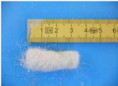
Photograph 1– [E] FKE –Reference for Fibre clumbs fibre = 30dtex-6mm
