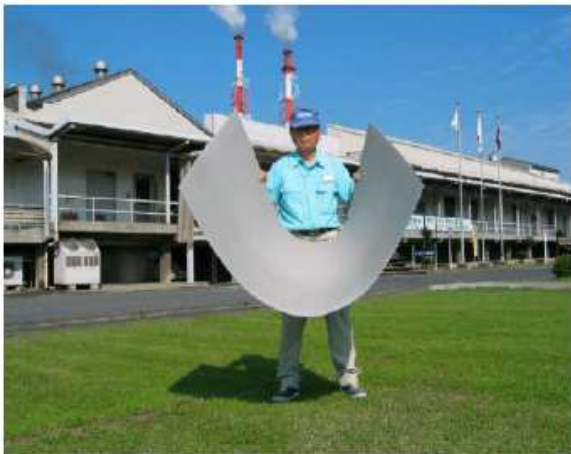
Figure 4 Bendable sheet (2mm thickness)
