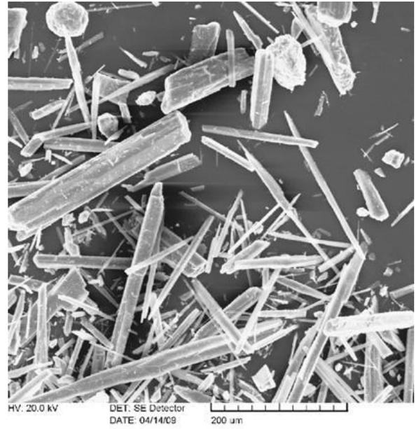
**Figure 9 – SEM picture of fibrous wollastonite particles**
