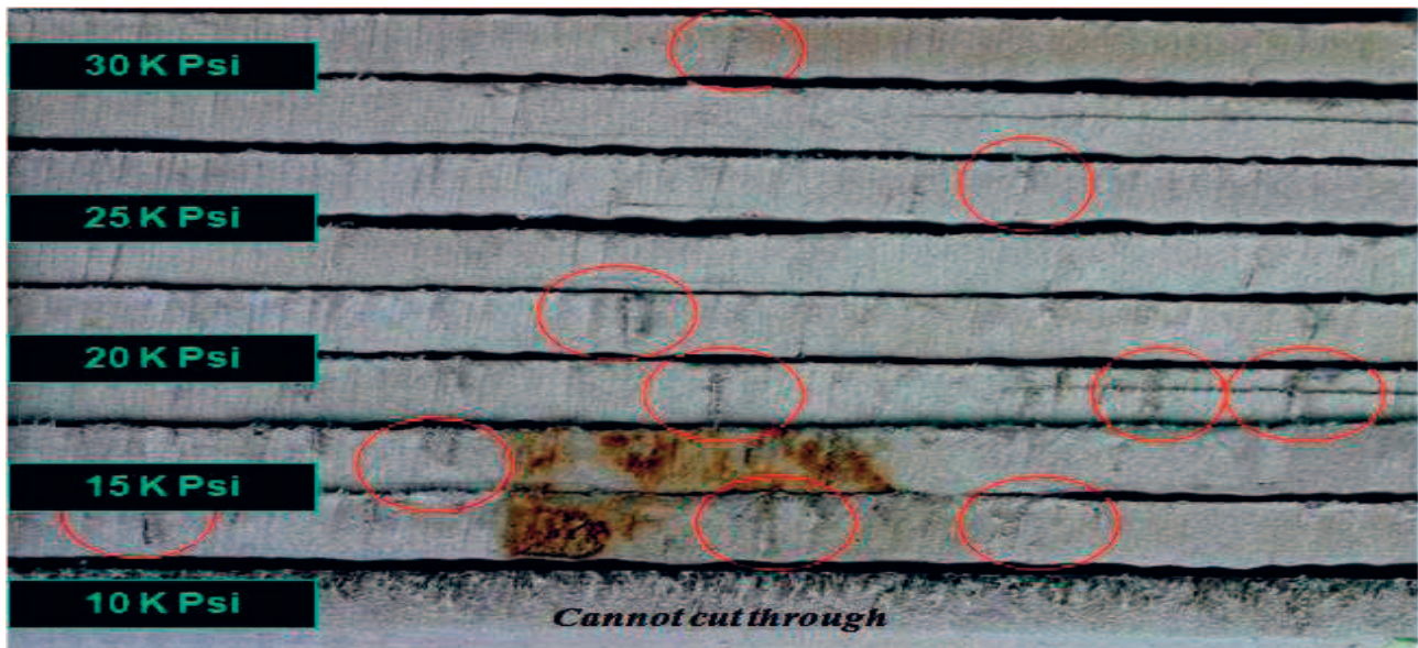
Figure 4 – Cut Edge Appearance – Effect of Working Pressure
