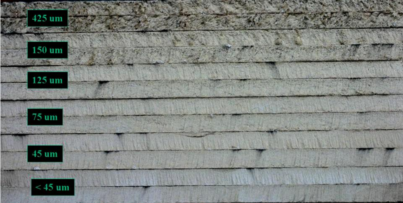
Figure 8 – Cut Edge Appearance – Effect of Sand Fineness
