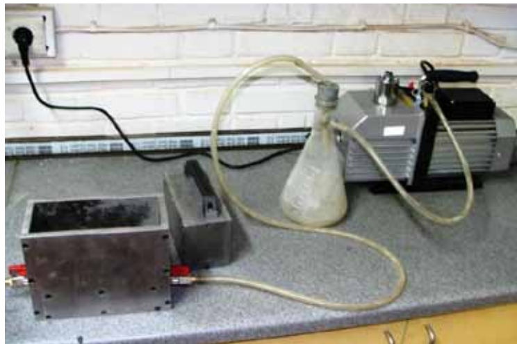
Figure 3: System set-up for making the specimens
