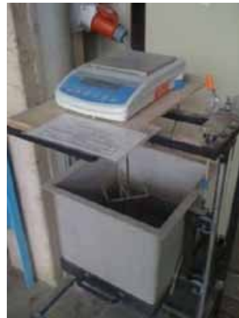
Figure 6. System set-up for finding the density of CCB
