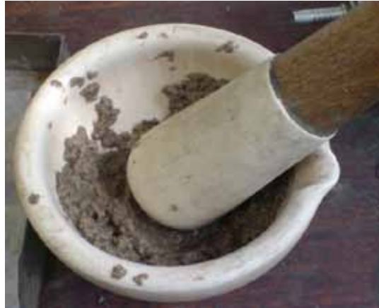
Figure 2 b : Beating cellulose fibres in the lab
