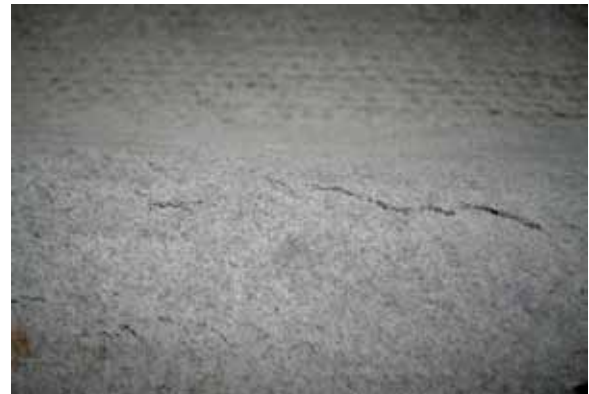
Figure 3 - Cracks on the PVA sheets
