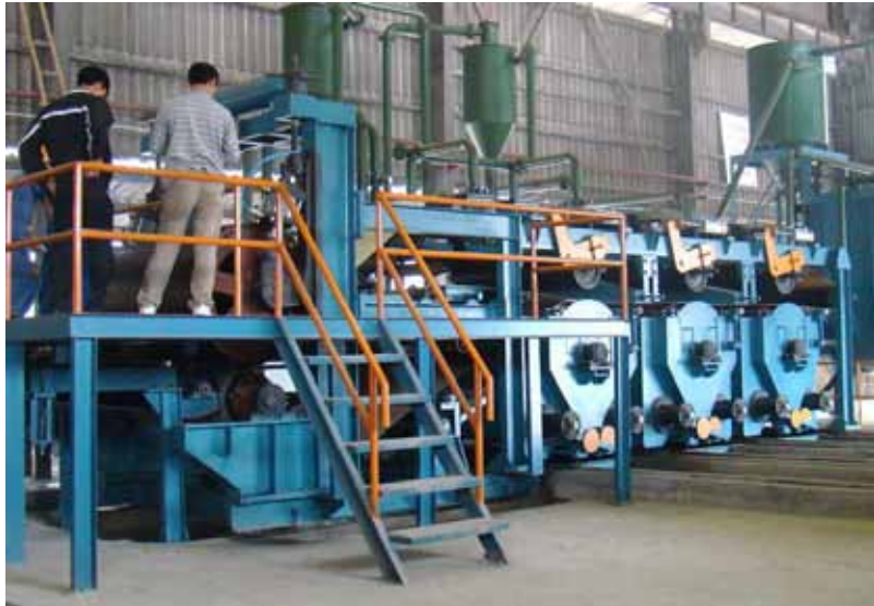
Figure 4 - A new Hatschek machine developed by RITM
