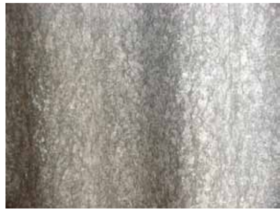
Figure 2 – Delaminating and fiber balling PVA cement products
