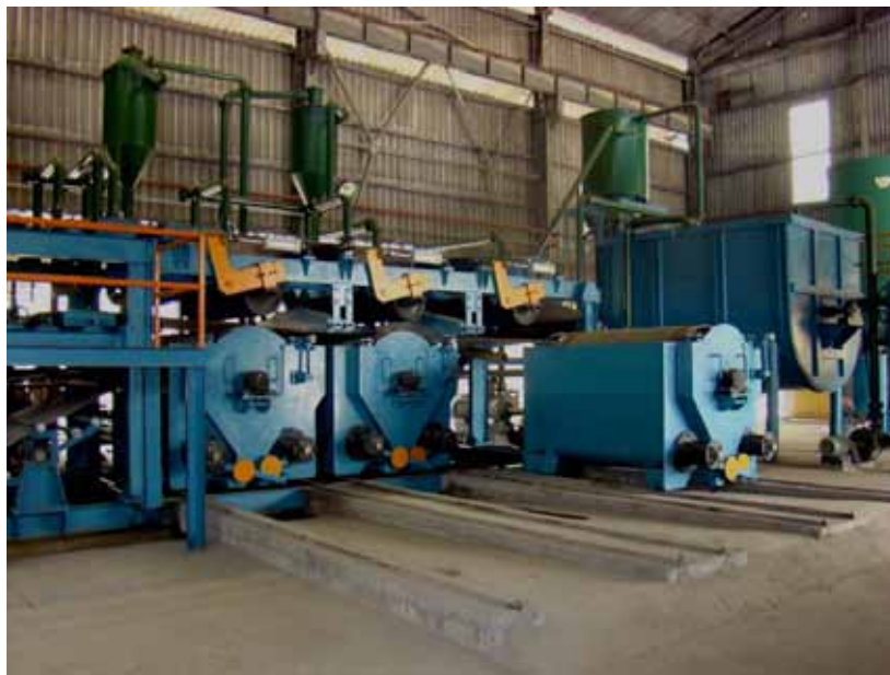
Figure 5 - Vat removing system of RITM Hatschek machine
