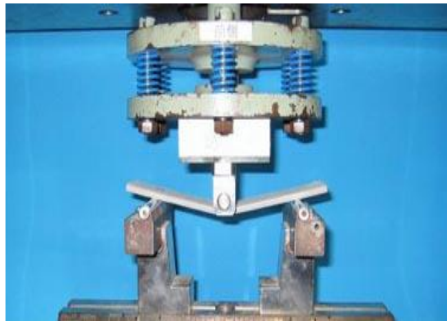
Figure 9 - Test set up for bending strength of PVA cement sheet
