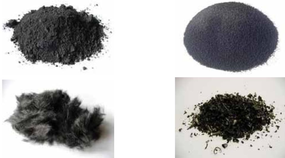
Figure 1 – Electrically conductive materials: micronized graphite, expanded graphite, carbon fibres, metal parings
