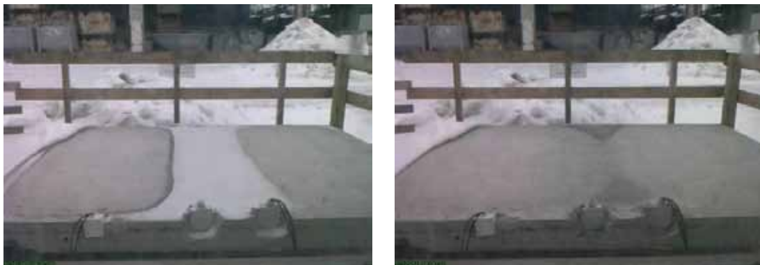
Figure 12 – Operation of the tempered panel in real conditions
