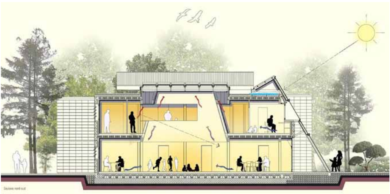
Figure 8 – Cross section of the building, showing the main passive devices for climate control.
