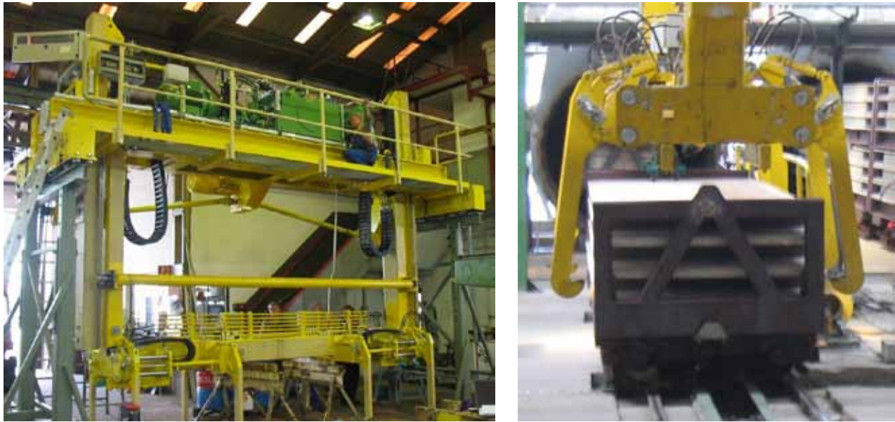
Figure 8 – WEHRHAHN loading machine during workshop assembly (left) and in operation (right)
