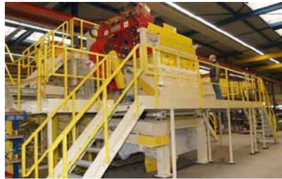
Figure 8 - Eltomatic CVS-16 Rotating Wood Wool Machine (cap.: 3.000 kg/hr.)
