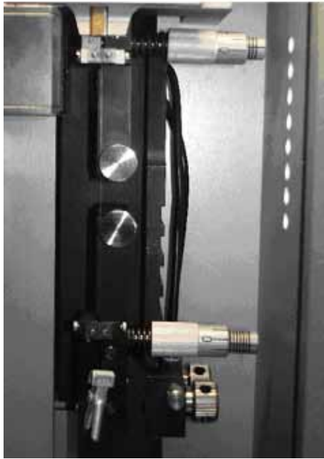
Picture 3: Wrap-bollard clamps for individual fibres
