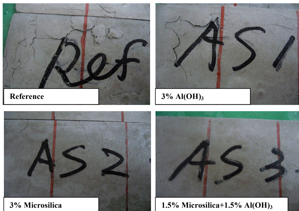
Figure 5 - Appearance of sample after 100 freeze-thaw cycles
