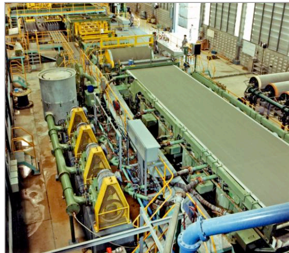
Figure 2 - Hatschek board machine
