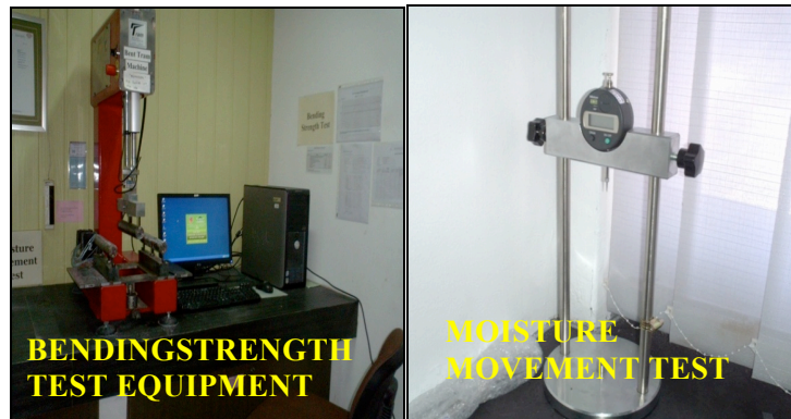
Figure 6 - Bending strength and moisture movement equipment
