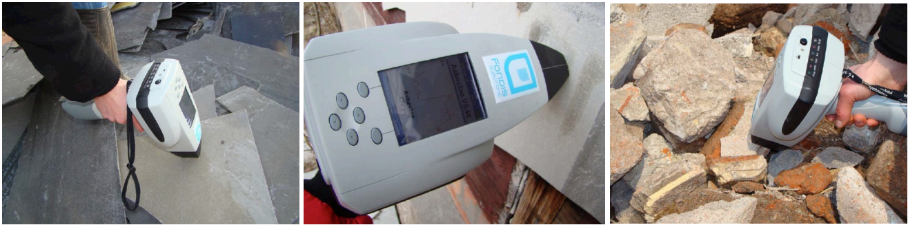
Figure 10 – Examples of in situ use of the NIR – based analysis tool
