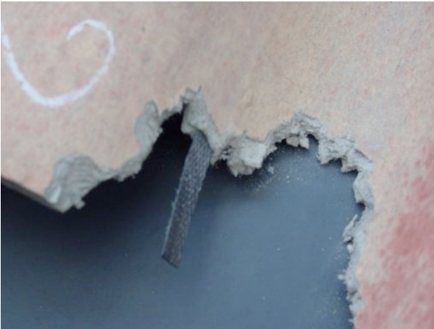
Close-up of partly liberated PP strip
