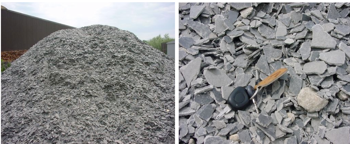
Figure 6 – Crushed FC slate waste as it is delivered to the clinker plant
