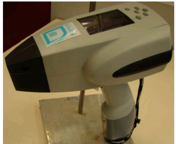
Figure 8 - NIR-Spectrum of a tissue containing > 40 % of chrysotile asbestos Figure 9 – The microPHAZIR analyser
