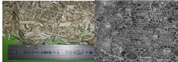
Figure 1 – Photography of raw shiv particles (left) SEM micrograph showing shiv micro-porosity (right)
