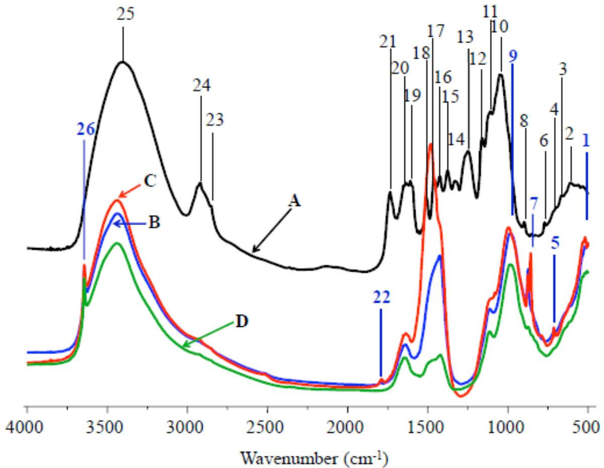
Figure 2 - FTIR spectra of (A) *Laccosperma secundiflorum*, (B) *L. secundiflorum*/cement mix, (C) *L. secundiflorum*/cement/ $\text{CaCl}_2$ , and (D) *L. secundiflorum*/cement/30 min cold water extraction. Each spectrum is an average of spectra from two specimens. Peak position and assignment as well as structural polymer for each peak are presented in Table 4.
