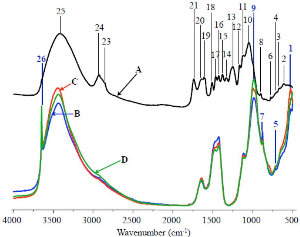
Figure 1 - FTIR spectra of (A) *Eremospatha macrocarpa*, (B) *E. macrocarpa*/cement mix, (C) *E. macrocarpa*/cement/ $\text{CaCl}_2$ , and (D) *E. macrocarpa*/cement/30 min cold water extraction. Each spectrum is an average of spectra from two specimens. Peak position and assignment as well as structural polymer for each peak are presented in Table 3.
