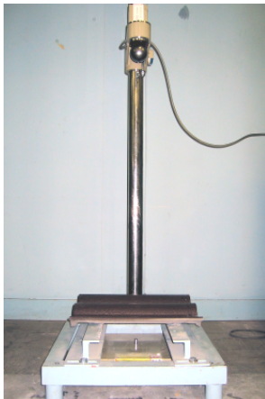
Figure 3 - Test method for evaluation item 4 (Falling ball test)
