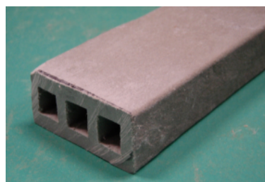
Figure 4 - Samples for evaluation item 1, 2, 3, 5 (Solid and Hollow extruded sheet)
