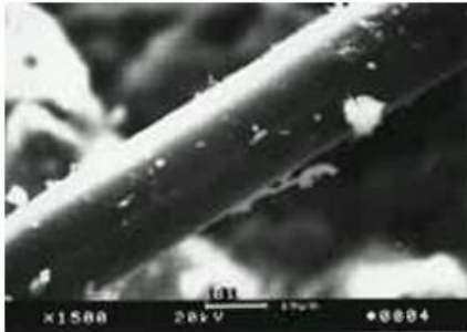
Photo 1 PVA Fibre surface Without microsilica
