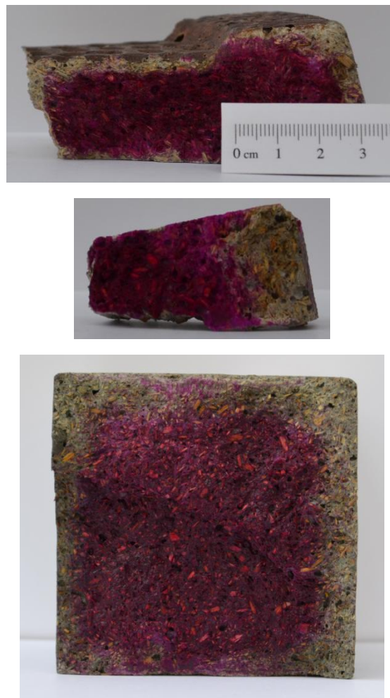
Figure 2. Carbonation of 4 years old outdoor WCC sample
