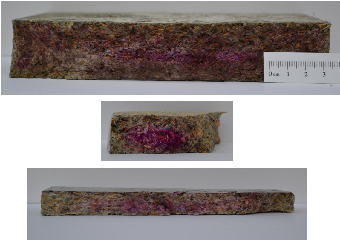
Figure 1. Carbonation of 4 years old indoor WCC samples
