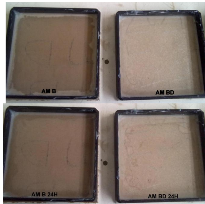
Figure 9 – Vertical Water Absorption Test
