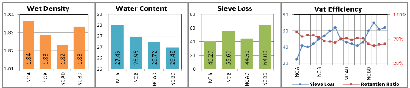
Figure 4 – Graph of Process data recorded during production of Natural Cured boards
