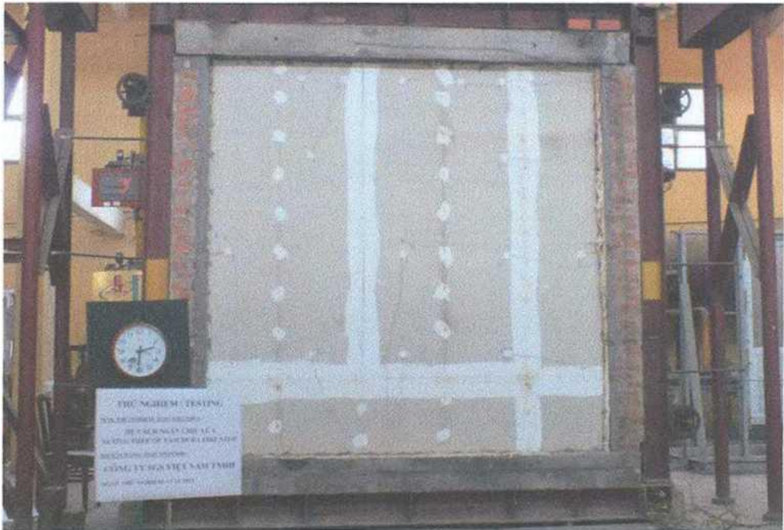
Figure 11: Specimen system after test (unexposed face)
