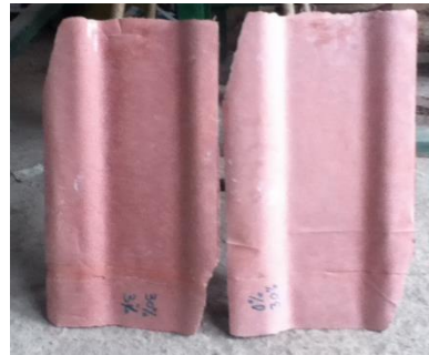
Figure 5: The Fully-Cured Roofing Tiles
