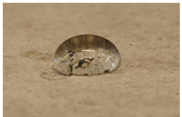
Figure 7: Picture showing a water droplet placed at the surface of a lab-made FRC boards modified with 0.25 % IE 6686 vs the dry weight of the board formulation.
