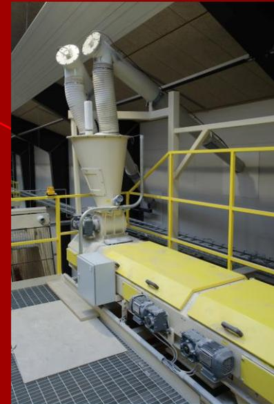
Cement and additives are precisely dosed into the mix
