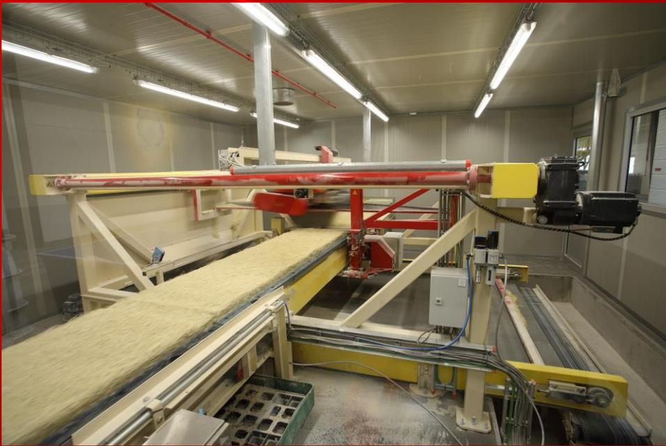
The fresh WWCB mat is cut into proper lengths, whereafter the moulds are stacked for transfer to the First Setting Area
