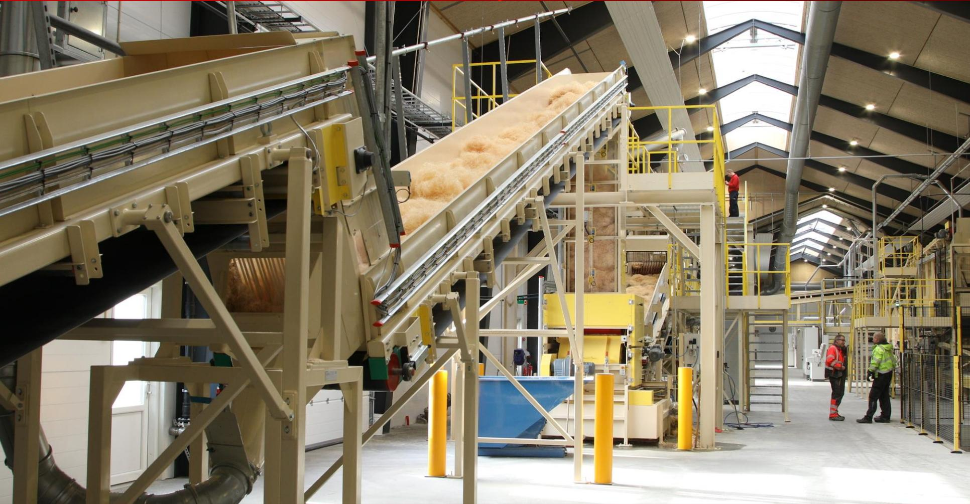
Wood Wool is transferred to the Mixing Group, where the proper amount of water, cement and additives will be added
